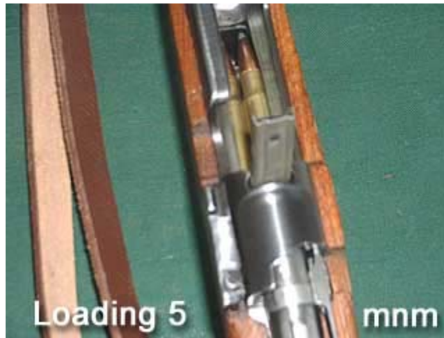
Loading 5 shows what the magazine looks like loaded with stripper clip still inserted.
