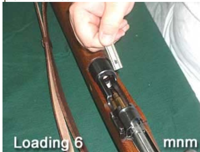
Pull stripper clip out of receiver as shown in Loading 6 . Close bolt (this action chambers first round into the chamber) and engage safety.
