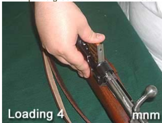
Once clip is inserted into receiver, push down on rounds until they strip off of clip and are loaded into the magazine as shown in Loading 4.
