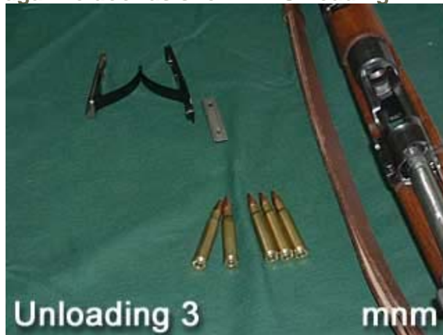
Allow all rounds in magazine to fall away from magazine. Safety Operations
