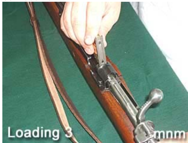
Push down on clip into grooves as shown in Loading 3.
