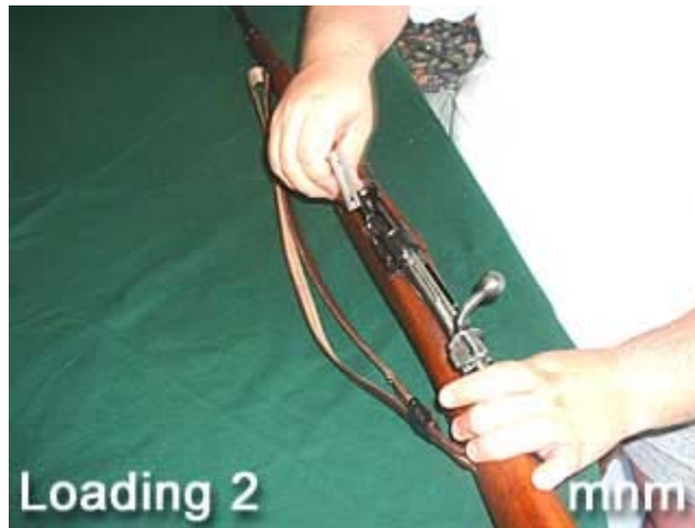
Open bolt and pull to rear of receiver. Place clip into guide in top of Mauser receiver.
