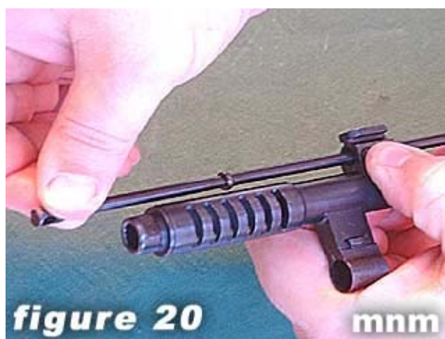
20) While depressing cleaning rod release button on bayonet lug , remove cleaning rod .
