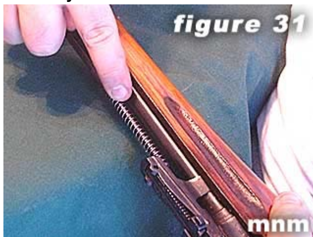
31) Remove the piston/rod assembly .
