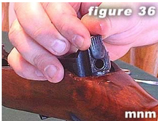
36) Rotate trigger release cover to expose trigger release.
