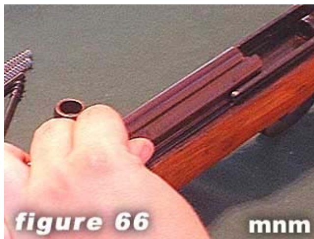
66) Replace bolt and bolt carrier into receiver.
