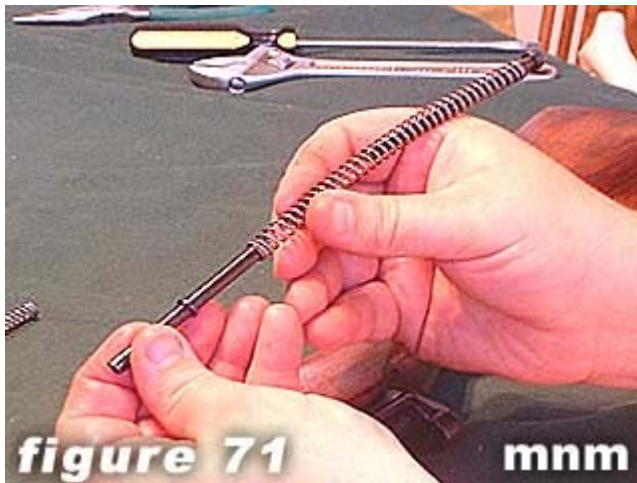
71) Attach rear recoil spring to middle spring guide .
