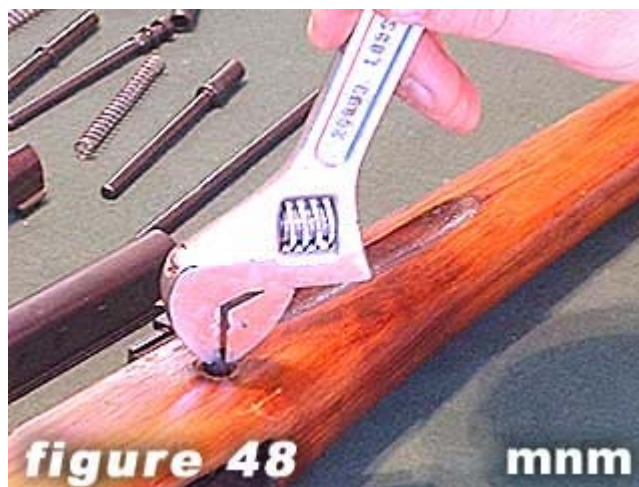
48) Tighten cross pin screw.
