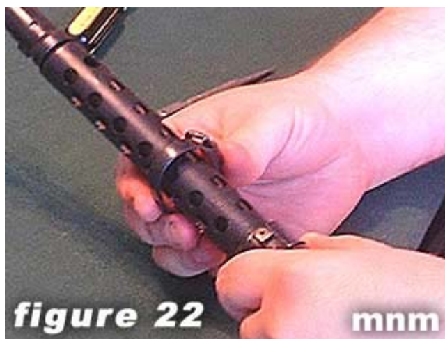
22) Slide the swivel band forward .
