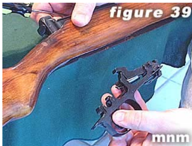
39) Figure 39 shows the removed trigger assembly .
