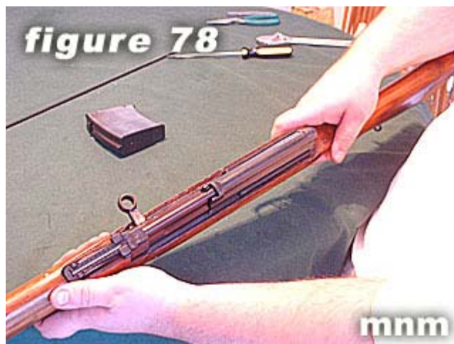
78) Figure 78 shows the reassembled receiver.
