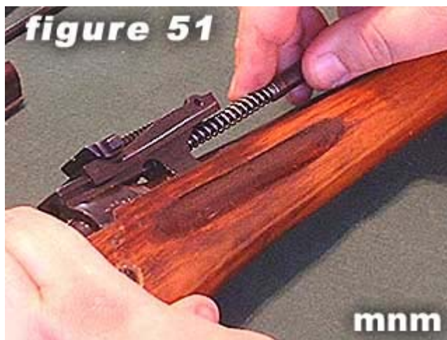
51) Insert piston rod extension and piston spring into rifle as shown in figure 51.
