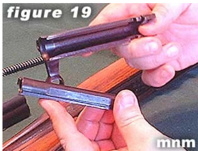
19) Figure 19 shows the separated bolt and bolt carrier .
