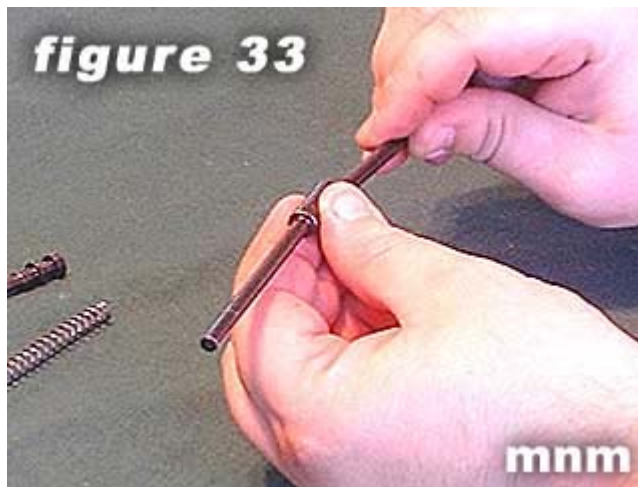
33) Remove the piston rod extension from piston rod.
