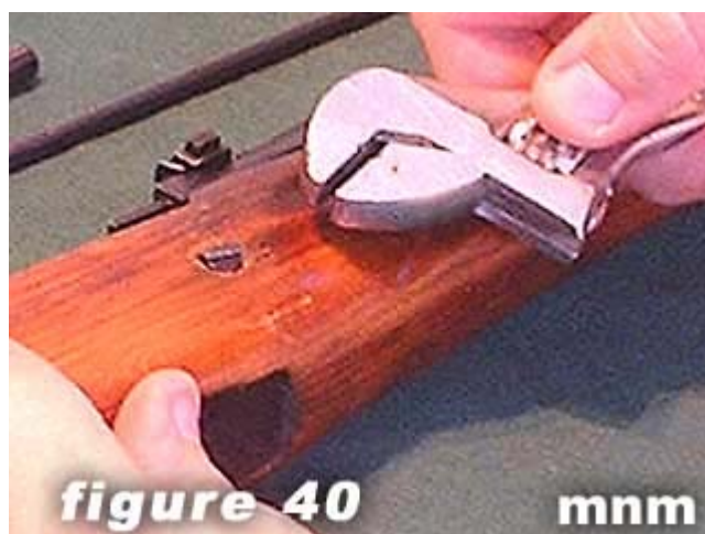
40) If you do not have an SVT tool you can if you are careful to not damage the stock use a pair of adjustable pliers to loosen and remove the cross pin screw .
