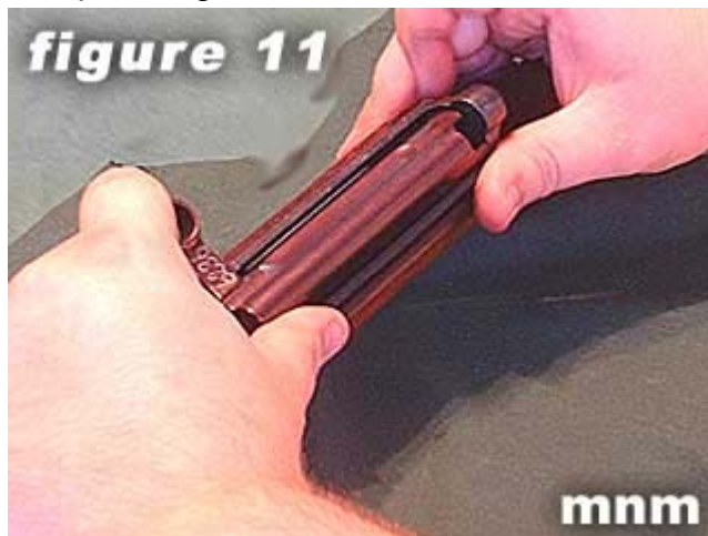
11) Pull bolt carrier to rear of receiver.
