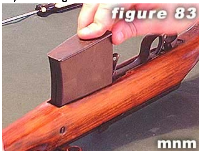
83) Lock magazine into place.
