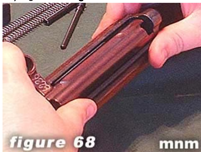
68) Pivot bolt carrier as show in figure 68 (bringing handle towards you). Lay bolt carrier down and into slot in receiver rails.
