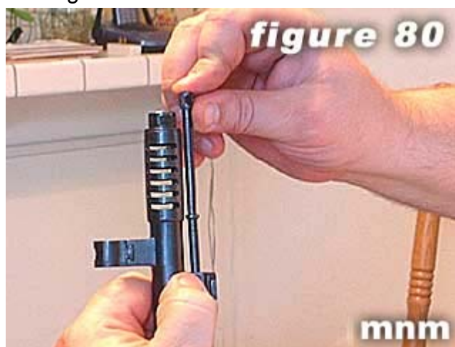
80) While depressing cleaning rod release button on bayonet lug , replace cleaning rod .
