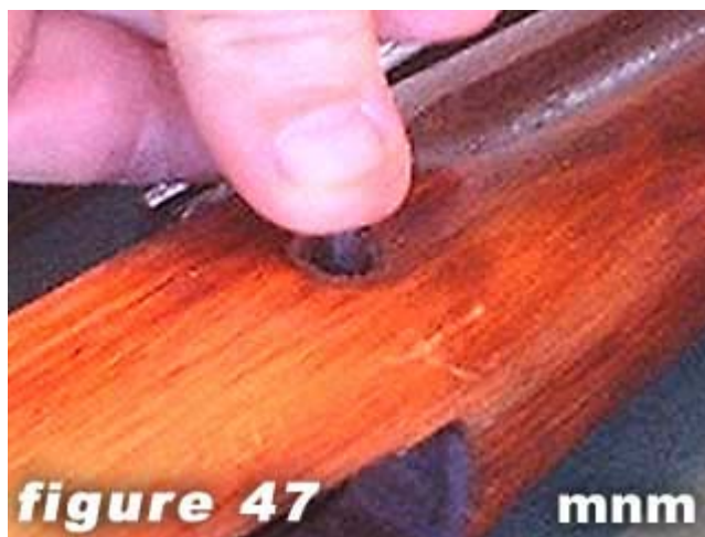
47) Install cross pin screw.
