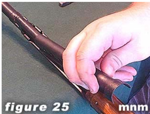
25) While lifting from rear, remove piston cover .
