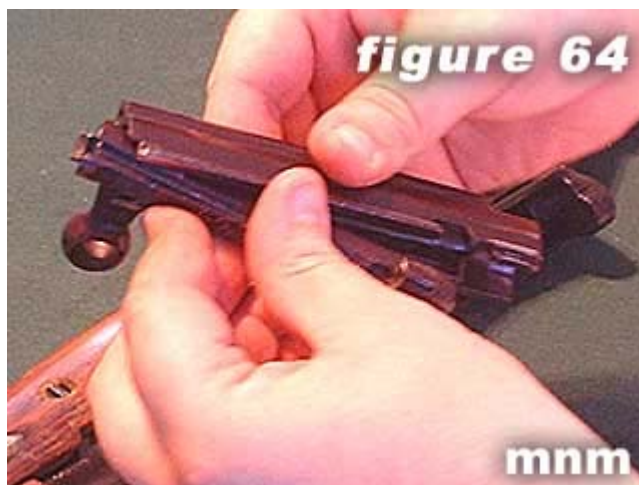
64) Combine bolt and bolt carrier.
