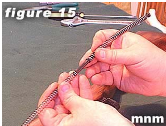
15) Remove front recoil spring from spring guide .
