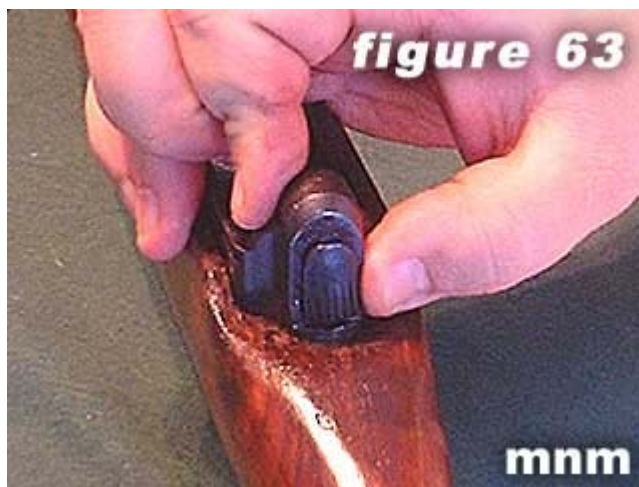
63) Rotate trigger release cover to cover trigger release.
