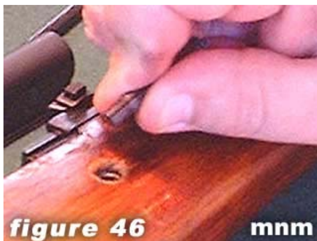
46) Compress cross pin screw as shown in figure 46.
