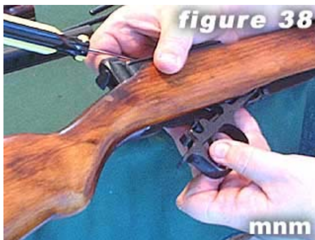
38) Trigger assembly can be removed as shown in figure 38.
