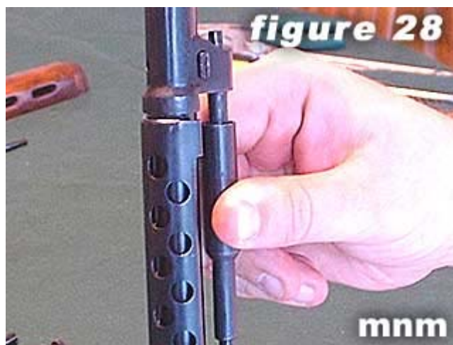
28) Slide piston cylinder down as shown in figure 28.
