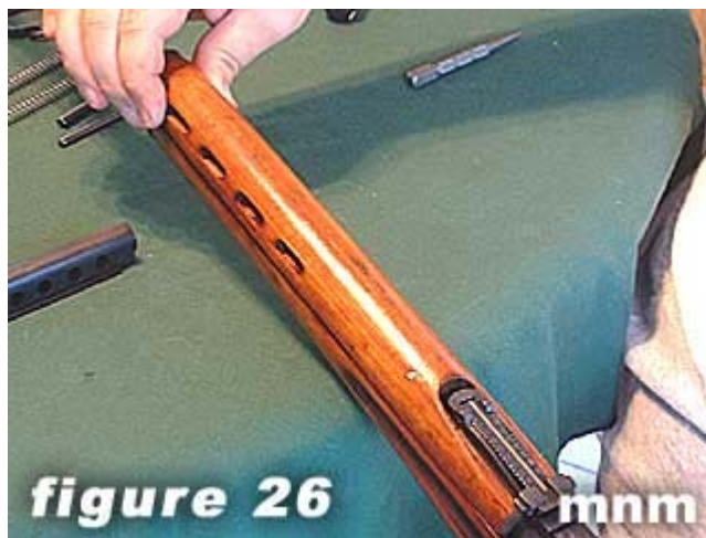
26) Lift hand guard from front.
