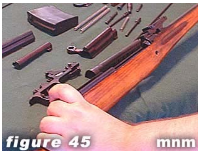
45) Return receiver and barrel assembly to stock.
