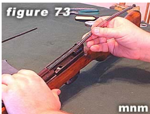
73) Slide front recoil spring into rear of bolt carrier .
