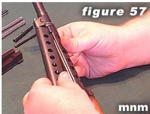
57) Replace piston cover . It slides under guides at front.
