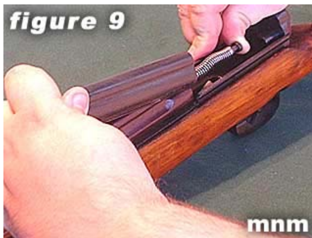
9) Remove receiver cover.
