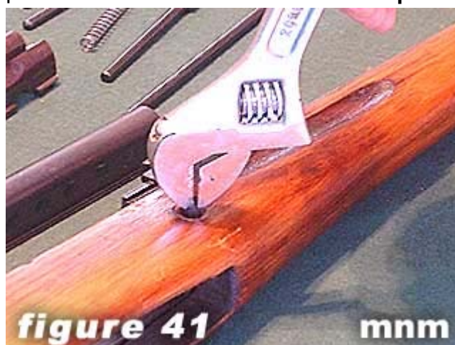
41) Turn cross pin screw counter-clockwise.
