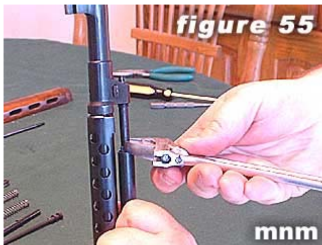
55) Turn gas piston clock-wise.
