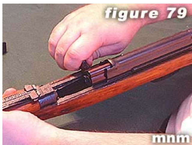
79) Cycle bolt carrier handle to make sure there is no binding.
