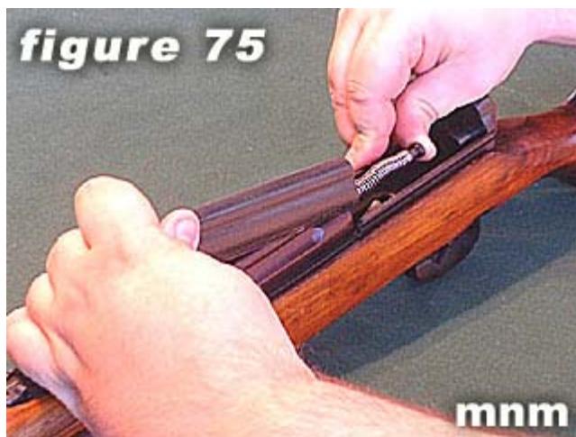
75) Compress recoil springs by pressing on rear spring guide . Place rear spring guide into slot inside rear of receiver cover .
