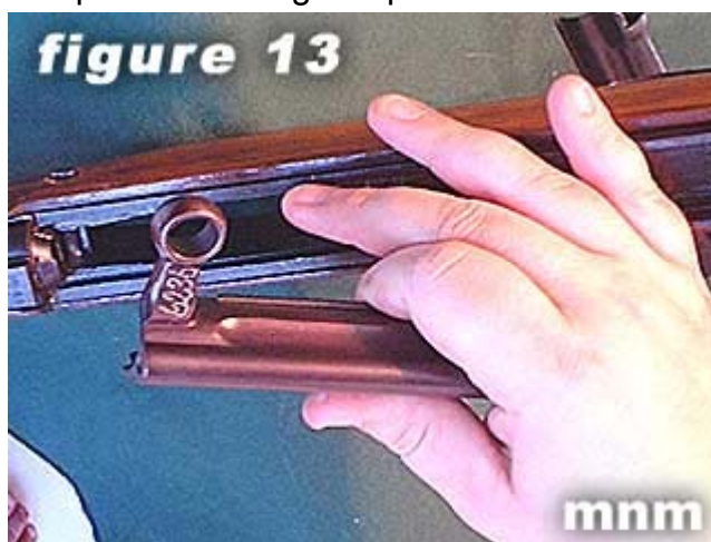
13) Remove the bolt carrier , bolt , and recoil spring assembly .
