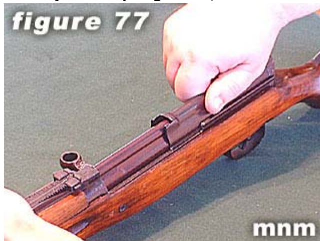
77) Allow receiver cover to slide into place.
