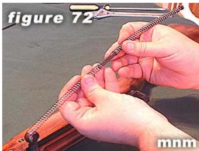
72) Attach front recoil spring to middle spring guide .
