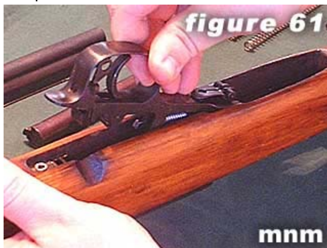
61) Reinstall trigger assembly .
