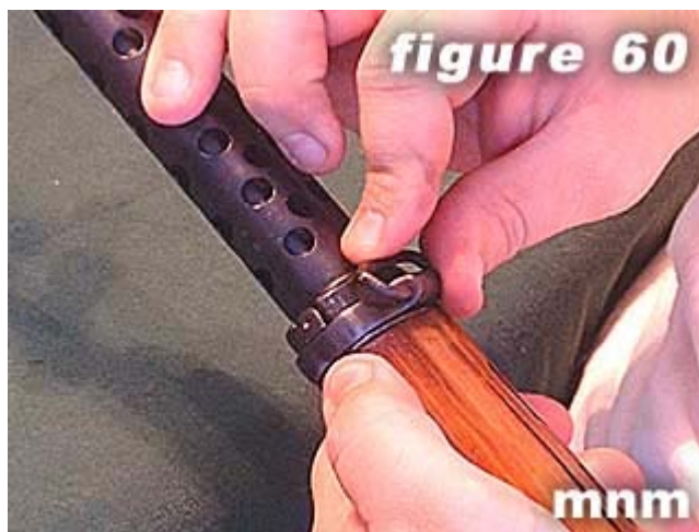
60) Depress swivel band spring and slide swivel band into place.
