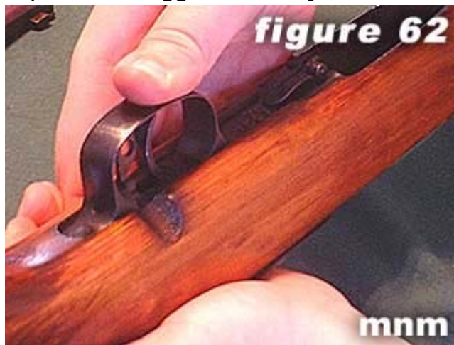
62) Depress trigger assembly and lock into place.
