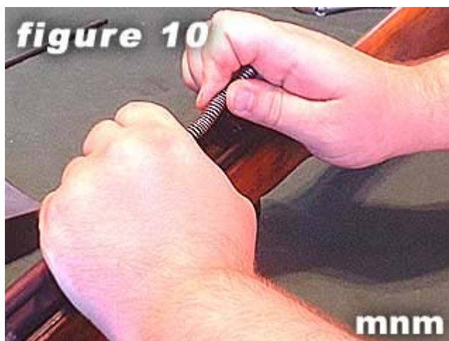
10) Allow rear spring and rear spring guide to expand and press against rear of receiver.
