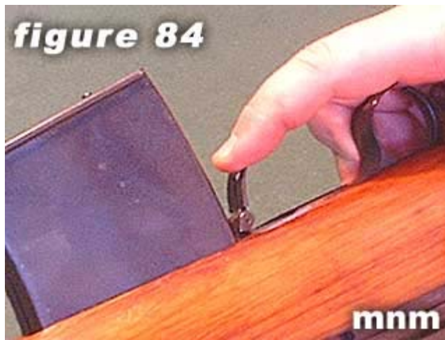
84) Depress magazine lever to rear.
