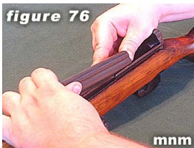
76) Slide receiver cover into slots and slide to rear while allowing recoil springs to expand.
