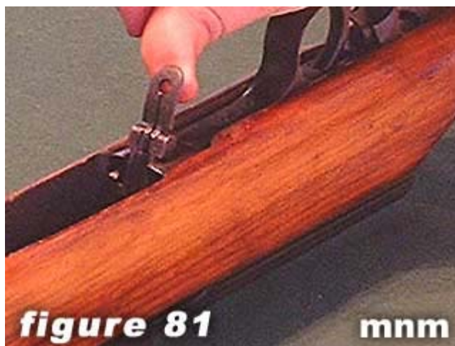
81) Lift magazine lever forward.
