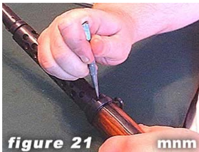
21) Depress swivel band spring .
