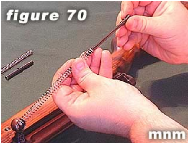
70) Replace rear recoil spring on rear spring guide .
