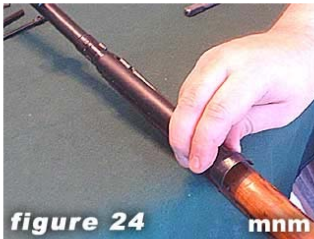
24) The piston cover is hinged at front.
