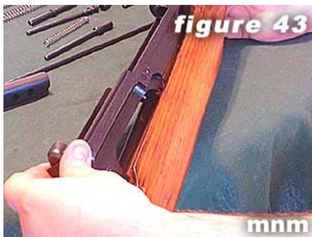
43) Lifting from rear remove receiver and barrel assembly and set aside.
