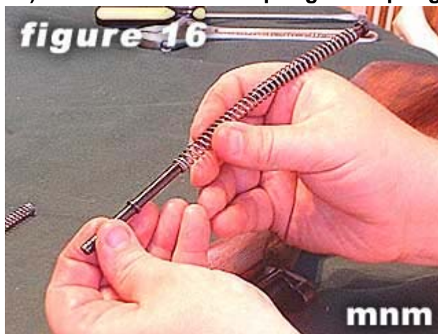
16) Remove rear recoil spring from spring guide .
