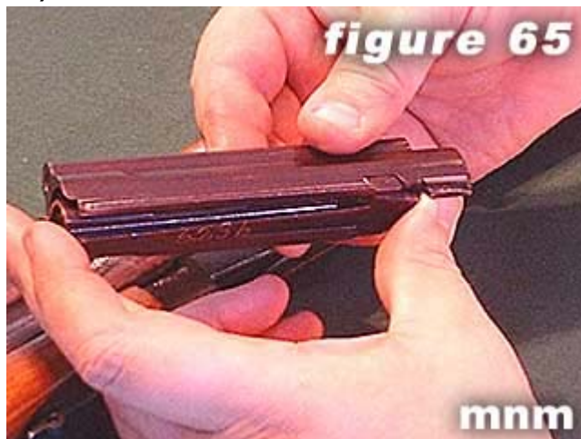
65) Bolt and bolt carrier fit together as shown in figure 65.
