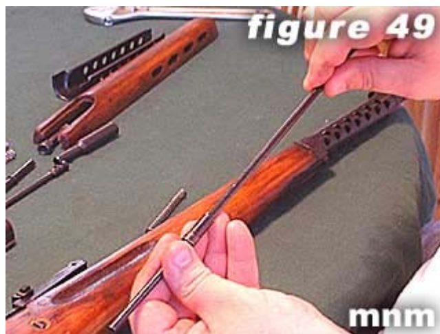
49) Place piston rod extension over piston rod.
