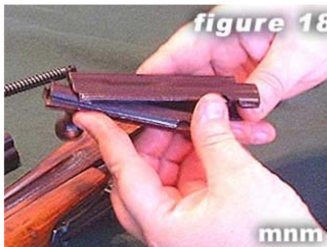
18) Separate bolt and bolt carrier .
