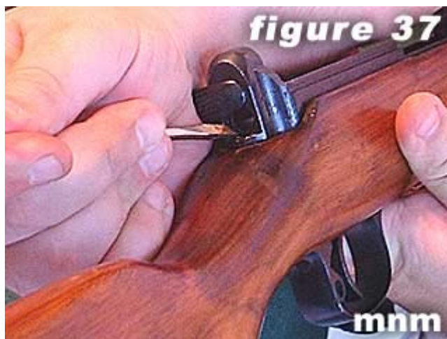
37) Depress trigger release.
