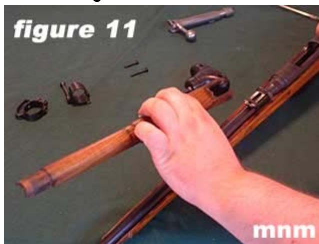
11) Remove the handguard and set aside.
