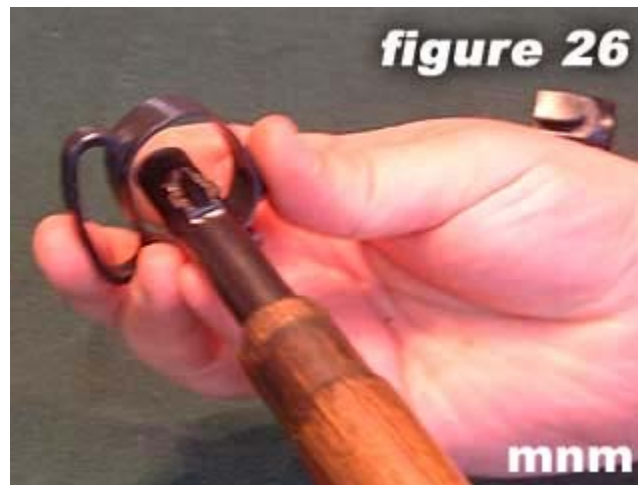
26) Slide the lower band back into place.
