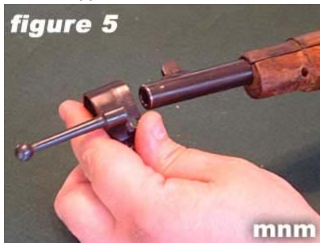
5) Slide the upper band forward.
