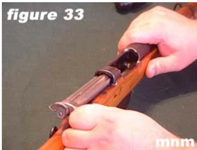
33) Reinsert bolt to receiver.
