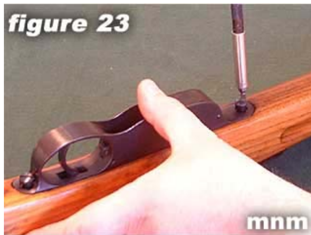
23) Tighten trigger guard front screw.
