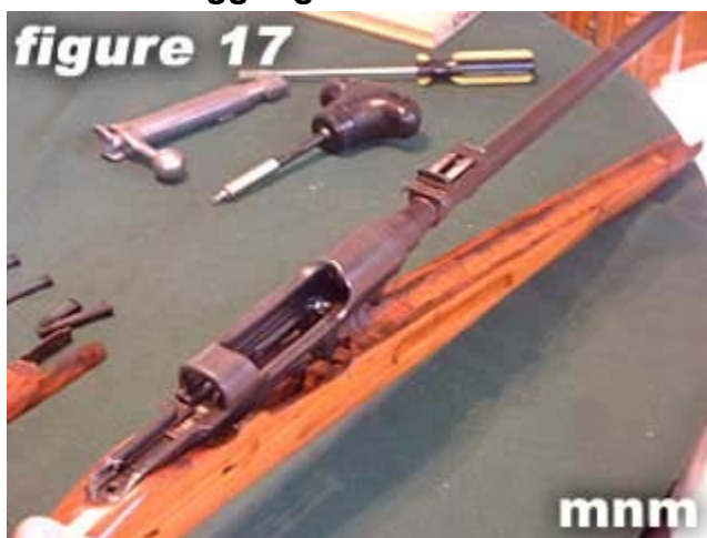
17) Remove the barrel and receiver assembly from the stock.
