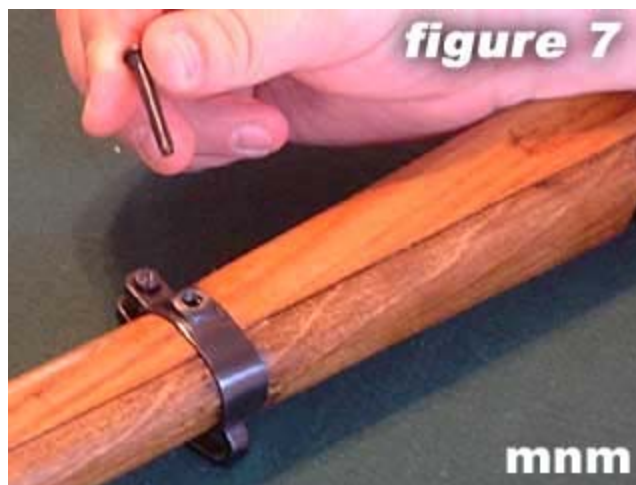
7) Remove lower band screw.
