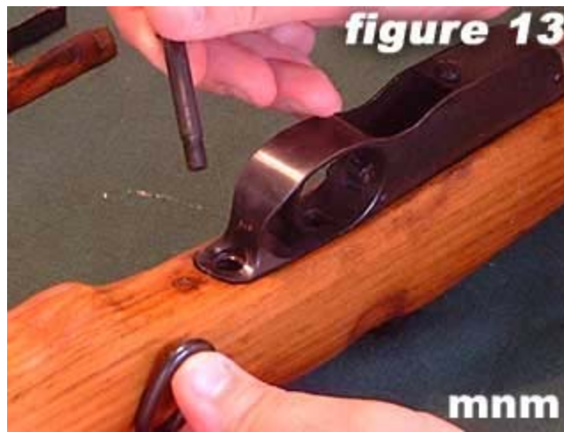
13) Remove the trigger guard rear screw .
