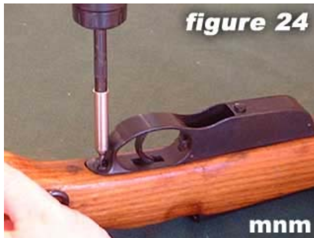
24) Tighten trigger guard rear screw.
