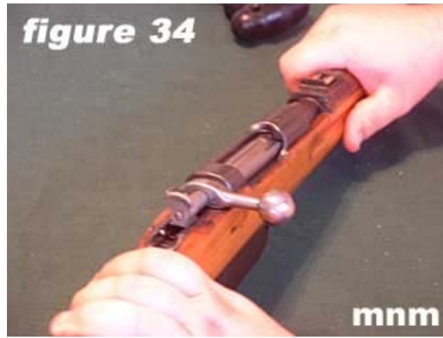
34) Push bolt forward and lock into closed position. Carbine is now reassembled.
