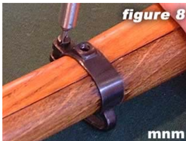
8) Loosen (only - do not remove) the lower band swivel screw.
