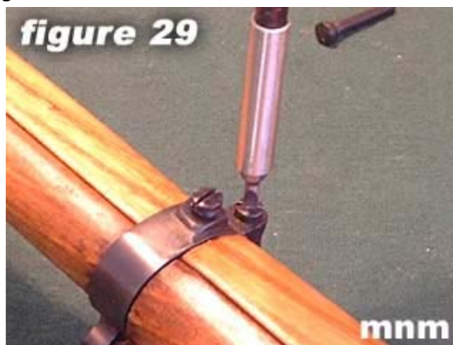
29) Tighten the lower band swivel screw .
