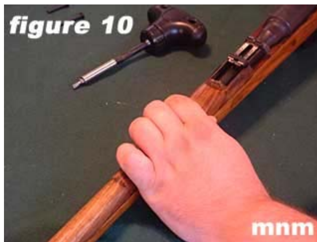
10) Slide the handguard forward.
