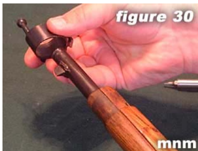
30) Slide the upper band back into place. Make sure bayonet lug is on bottom.
