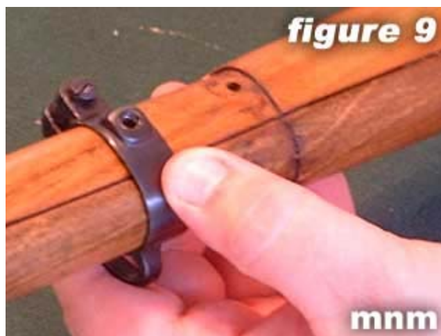
9) Slide lower band forward.
