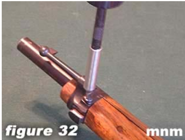
32) Tighten the upper band screw.
