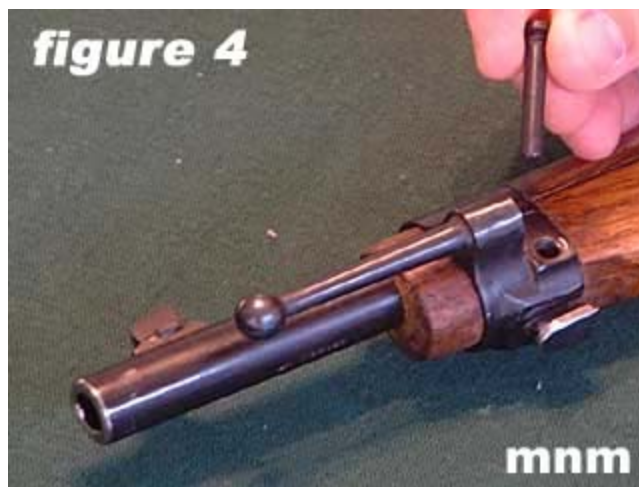
4) Remove the upper band screw .
