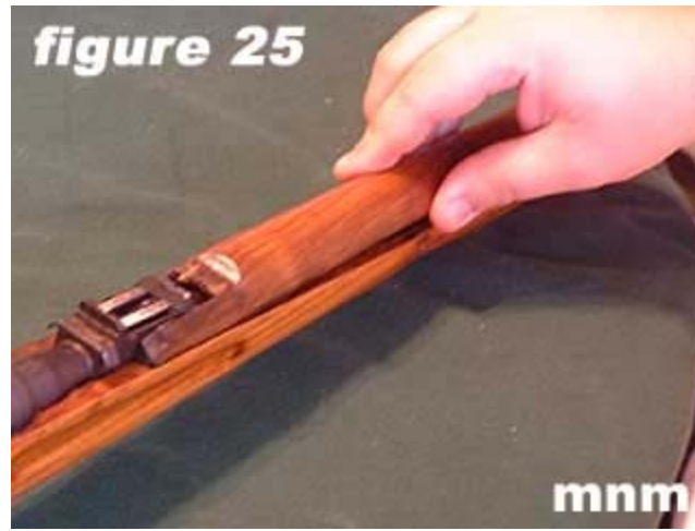
25) Slide the handguard to the rear (as shown in figure 29 ).
