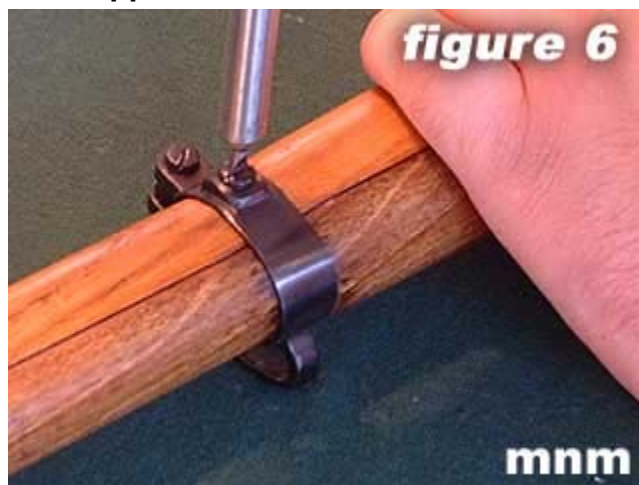
6) Loosen lower band screw .
