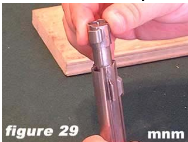
29) Push bolt head about midway into bolt body (as shown in figure 29 ).
