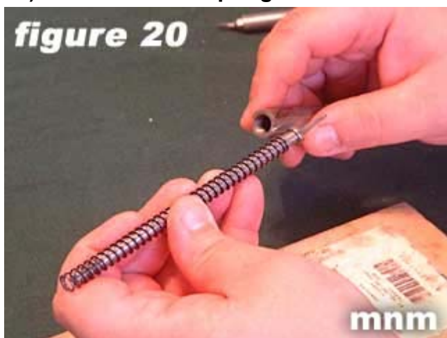
20) Remove striker spring and striker from bolt head .
