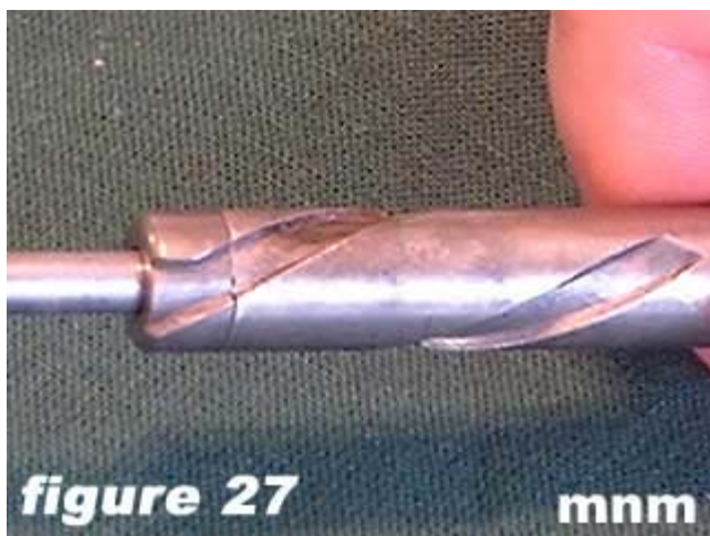
27) Figure 27 shows how the striker spring retainer and bolt head flutes should be aligned.
