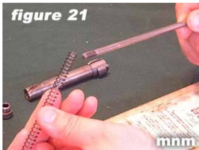
21) Separate striker spring from striker .
