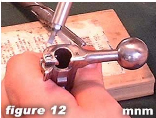
12) The safety lever is held in place by the safety screw (as shown in figure 12 ).
