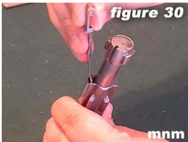
30) Insert extractor (as shown in figure 30 ) into channel in bolt body .
