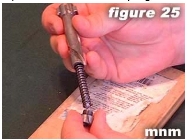
25) Return striker spring retainer and compress striker spring .
