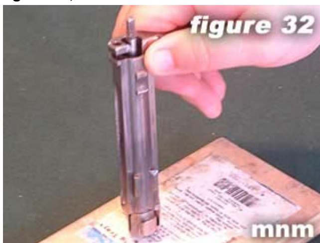
32) Place the bolt face against a block of wood and depress until the rear of the striker is fully extended to the rear.
