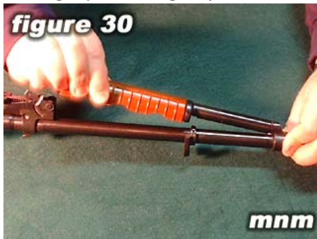
30) Attach the gas cylinder tube to gas cylinder (as shown in figure 30 ).
