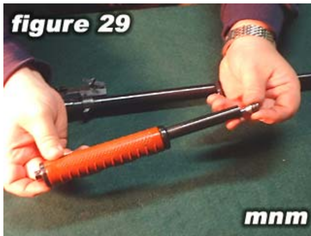
29) Place the gas piston into gas cylinder tube .
