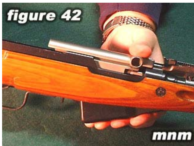
42) Slide the bolt and bolt carrier towards the front of receiver .
