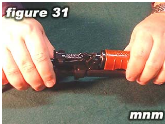
31) Make sure the end of the piston rod is flush with the end of the gas cylinder tube and then snap in down and into place (as shown in figure 31 ).
