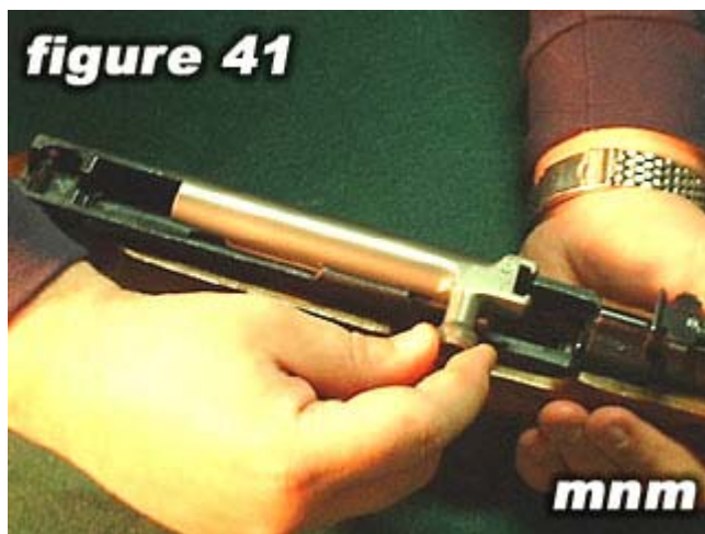
41) Install the bolt and bolt carrier into rear of receiver .
