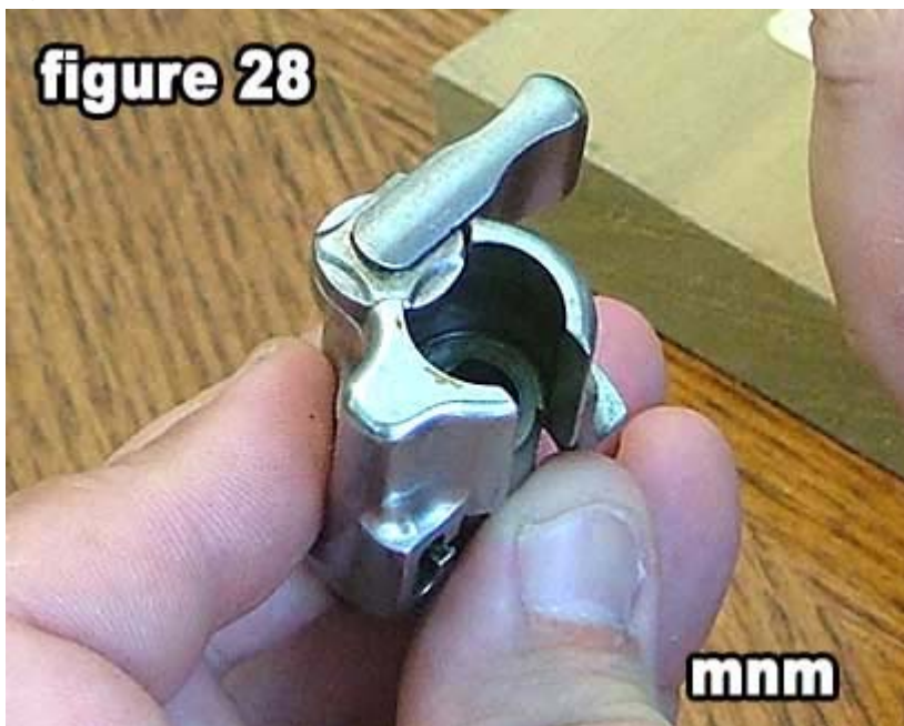
28) Figure 28 shows the safety properly installed.
