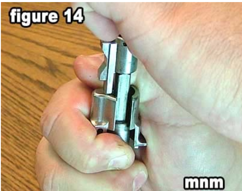
14) Turn cocking sleeve 1/4 turn in either direction.
