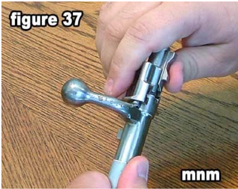
37) Rotate the bolt sleeve clockwise.
