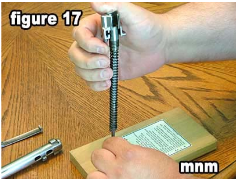
17) Allow main spring to fully expand as shown in Figure 17.
