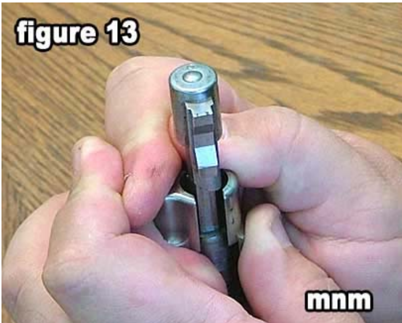
13) Slide the bolt sleeve until the cocking sleeve clears and can be turned in either direction.
