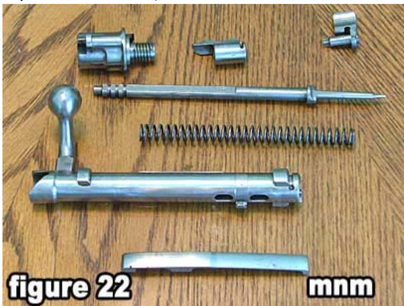
22) Figure 22 shows the completed Mauser bolt disassembly.
