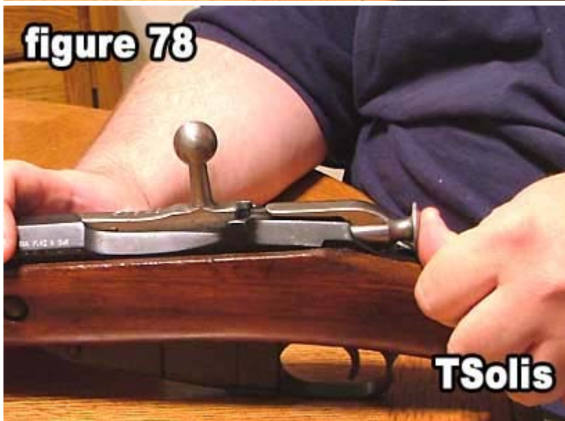
78) Push the bolt fully forward.
