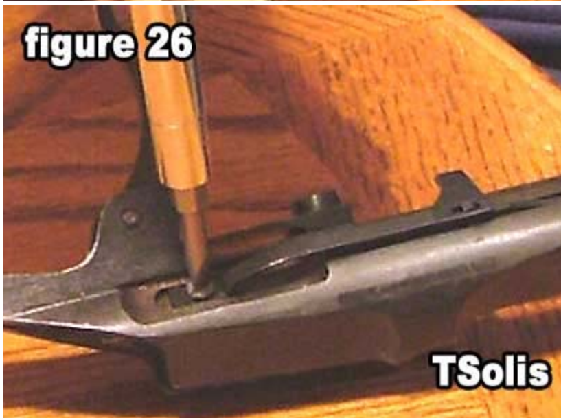
26) Unscrew the ejector screw.
