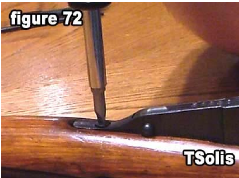
72) Tighten the trigger guard screw.
