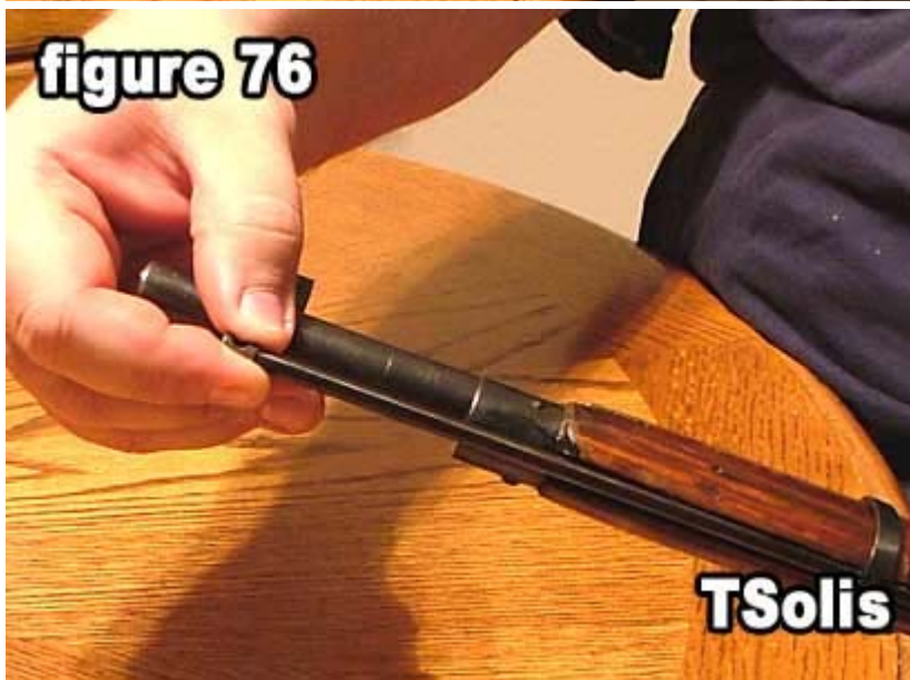
76) Tighten the cleaning rod.
