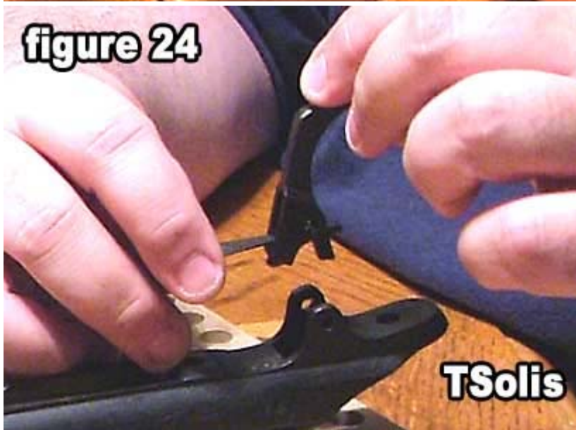
24) Remove the trigger and bolt stop.
