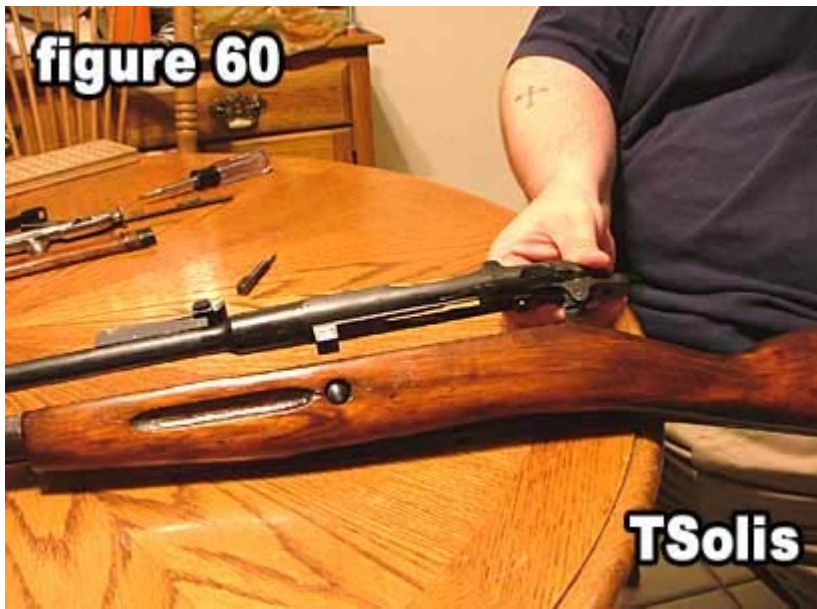
60) Insert the barrel and receiver into the stock.
