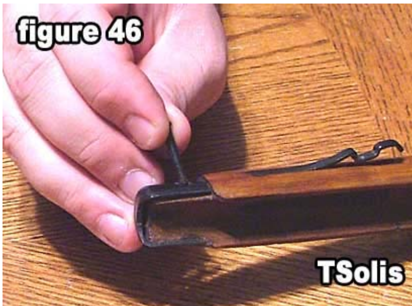
46) Insert the nose cap screw.
