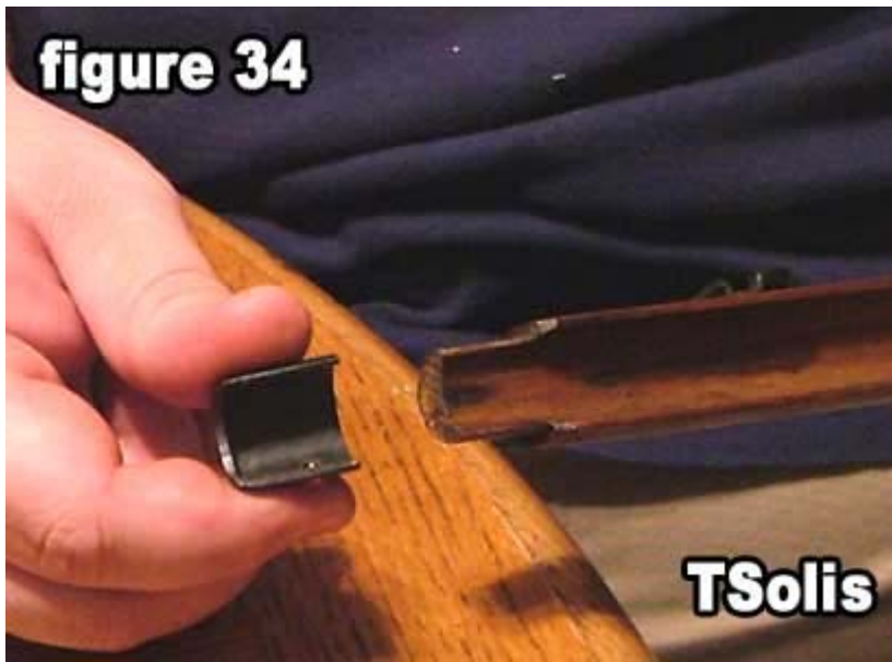
34) Remove the stock nose cap.
