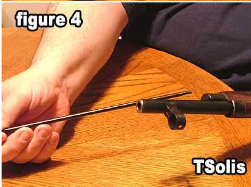
4) Remove the cleaning rod.
