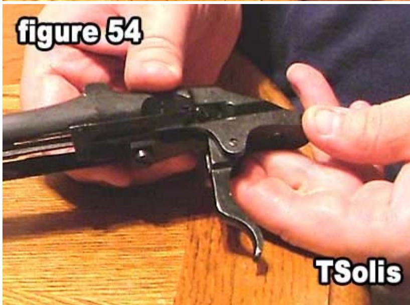
54) Figure 54 shows the correctly assembled trigger assembly.
