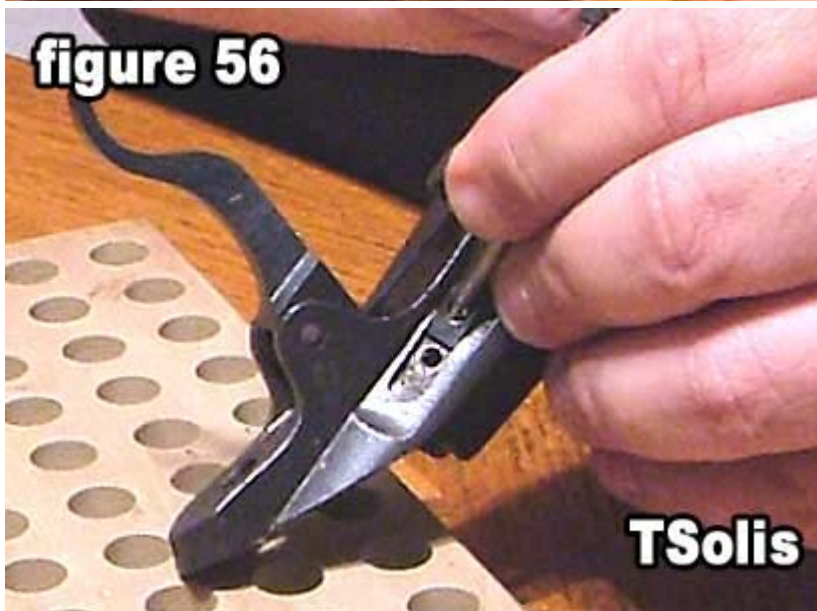
56) Slide the ejector spring into the slot.
