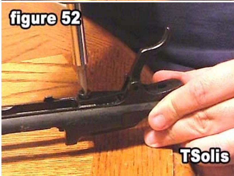
52) Tighten the bolt stop screw.
