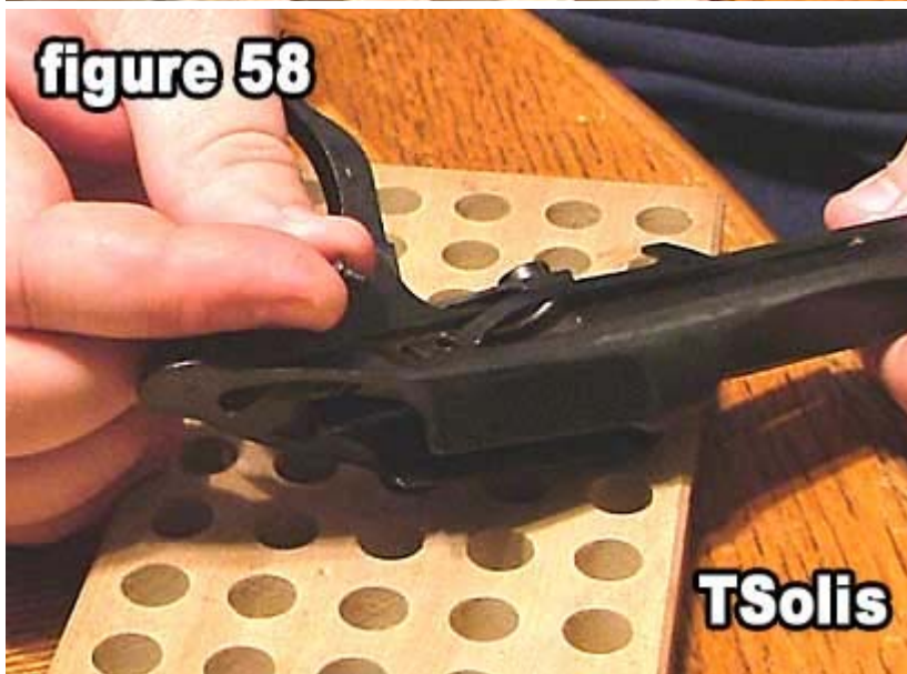
58) Insert the ejector spring screw.
