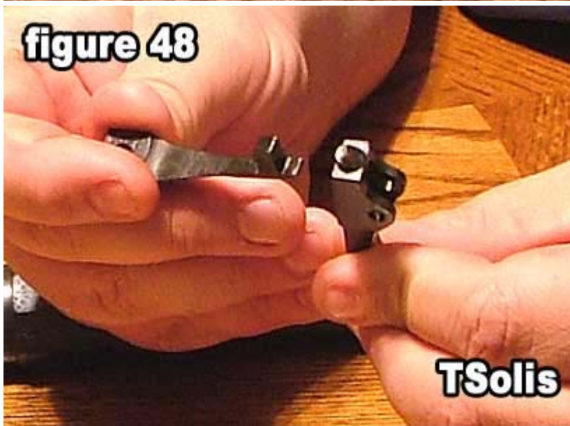
48) Combine the trigger and bolt stop as shown in figure 48.
