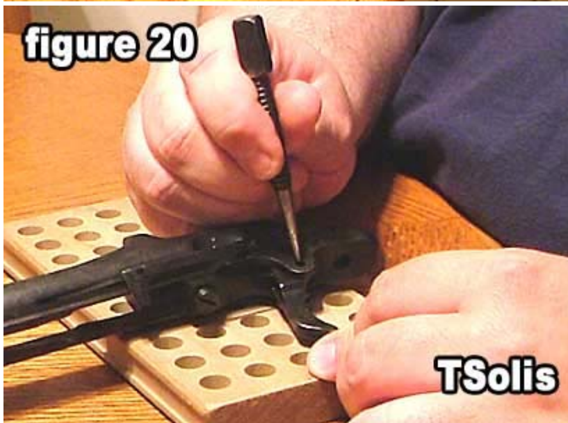
20) Using a pointed object push the trigger pin out of the trigger.
