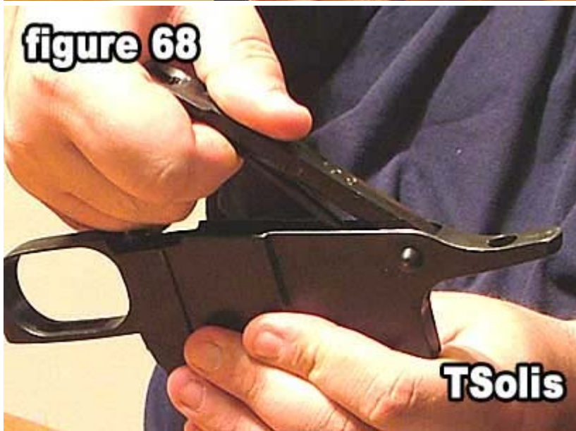
68) Replace the magazine follower and floor plate assembly in the magazine.
