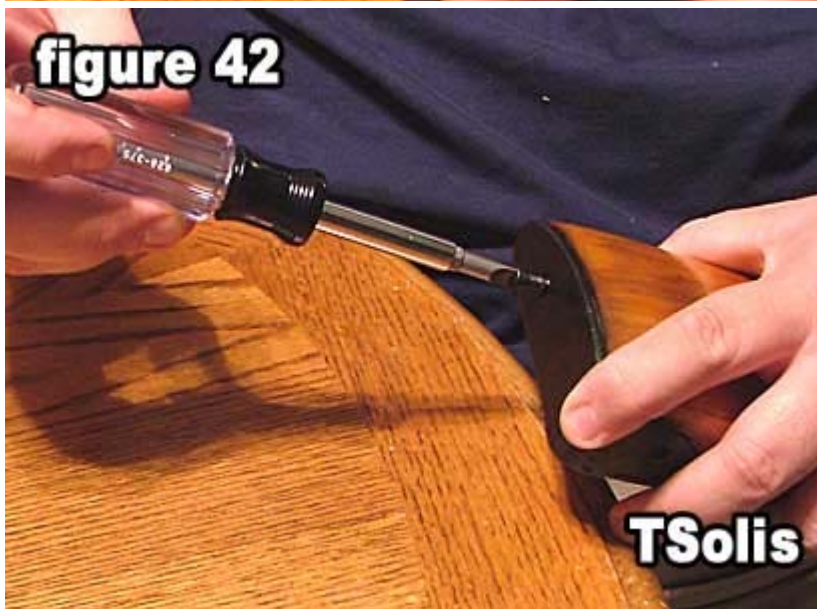
42) Tighten the lower butt plate screw.
