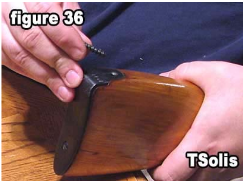
36) Remove the upper butt plate screw.
