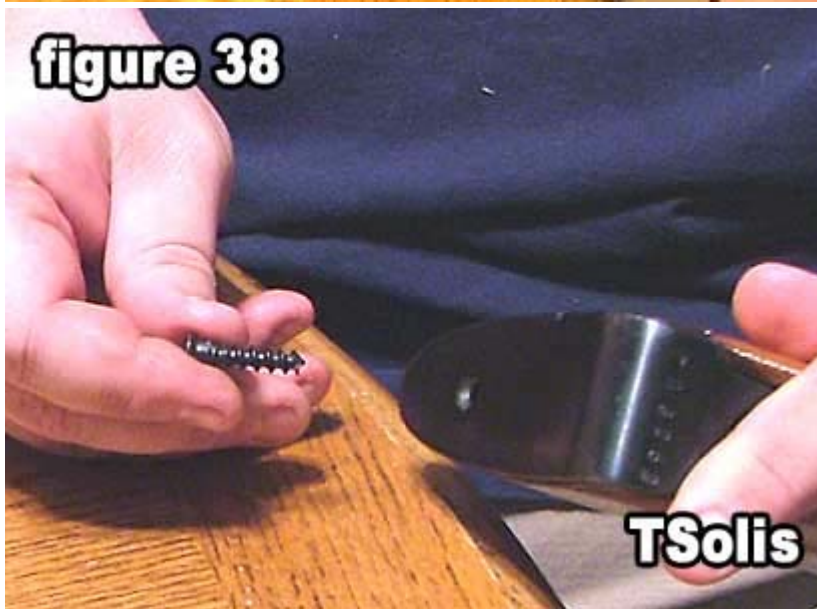
38) Remove the lower butt plate screw.
