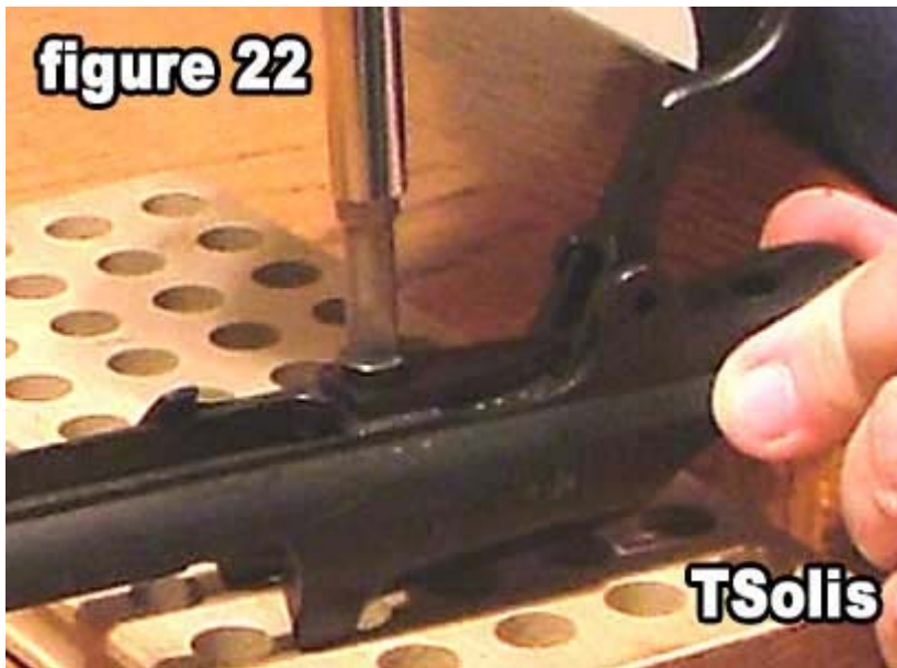
22) Unscrew the bolt stop screw.
