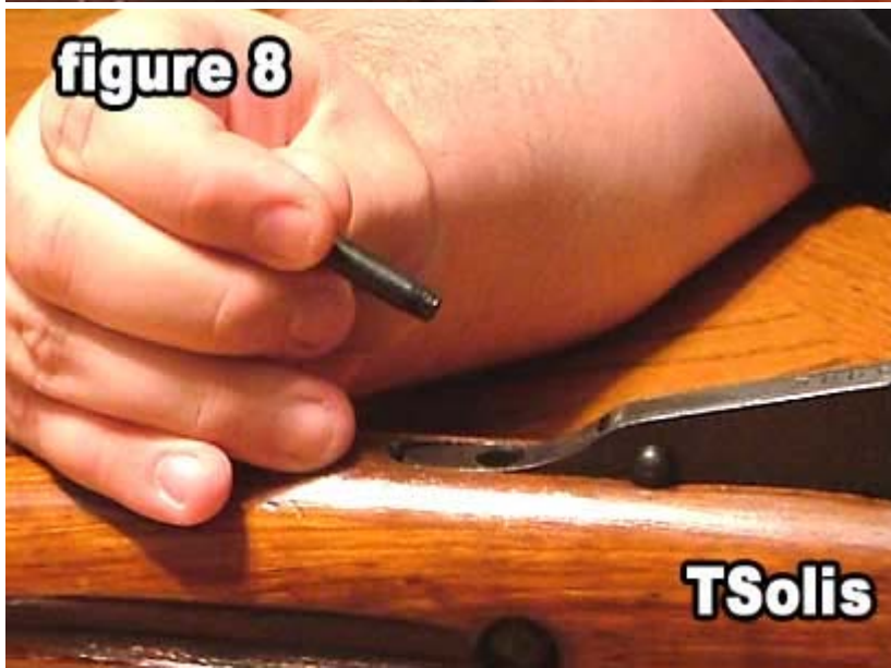
8) Remove the trigger guard screw.
