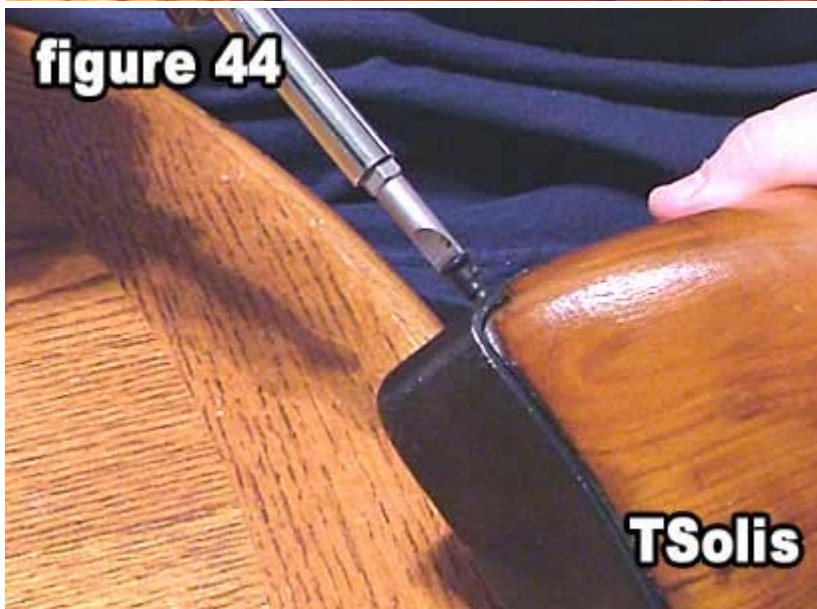
44) Tighten the upper butt plate screw.
