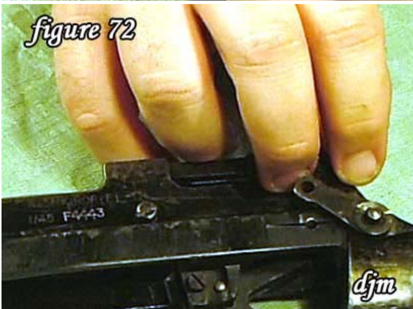
72) Install the locking bolt and safety catch.
