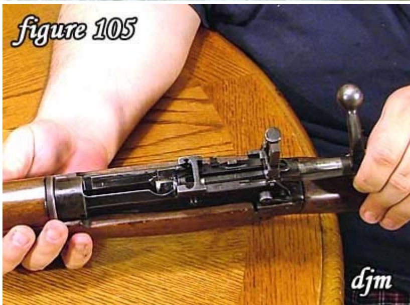
105) Slide the bolt fully forward.
