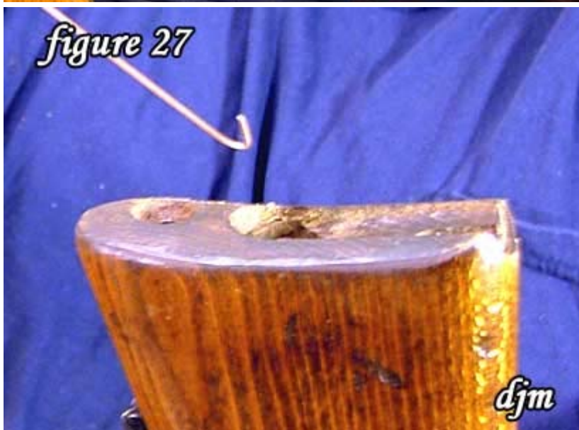
27) Remove felt wad with a cut-off clothes hanger (as shown in figure 27).
