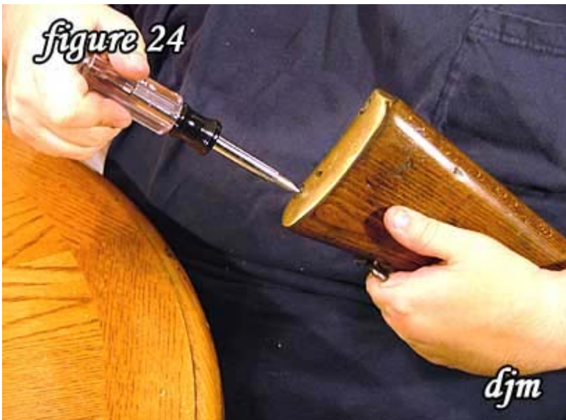
24) Loosen the butt plate screws.
