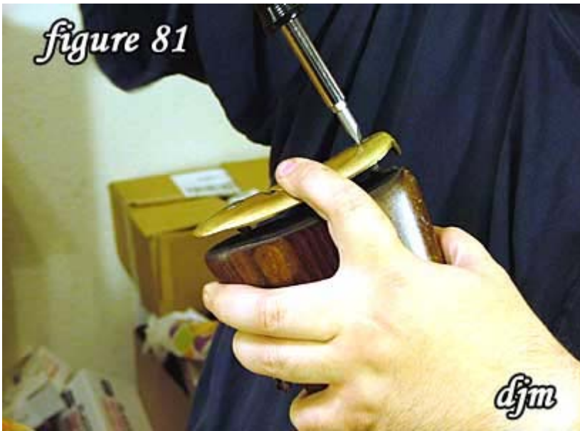
81) Tighten both butt plate screws.
