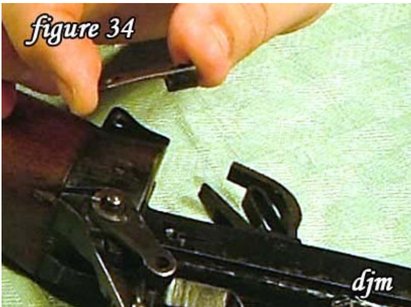
34) Remove the locking bolt spring.
