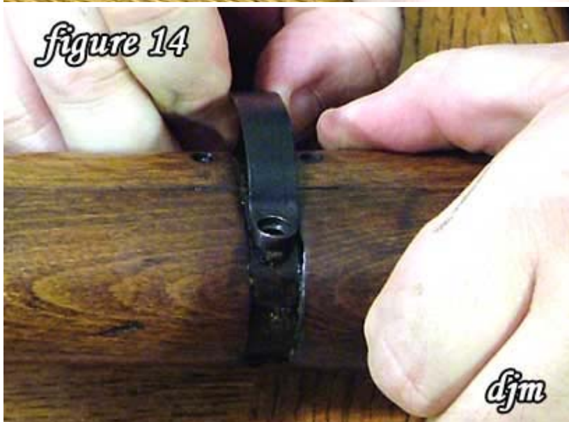
14) Spread slightly the lower band and remove from the stock.
