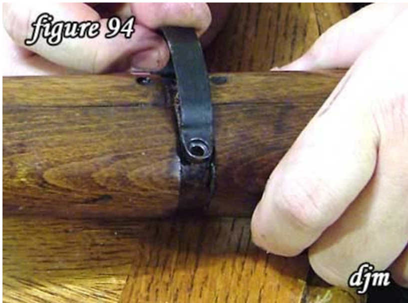
94) Spread slightly the lower band and replace on the stock.
