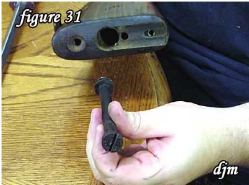
31) Figure 31 shows the stock bolt.
