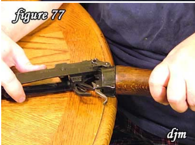
77) Reinsert butt stock into butt socket.
