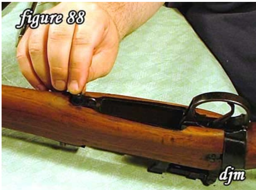
88) Reinstall the front trigger guard screw.
