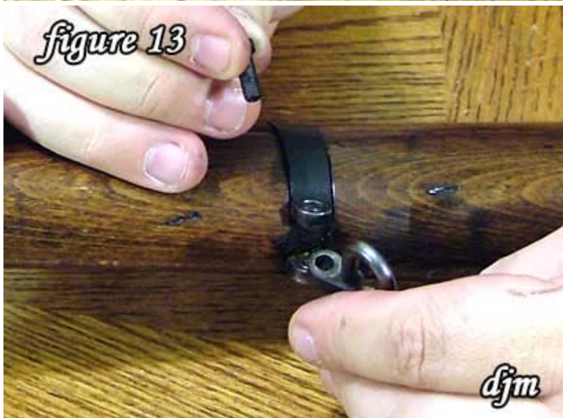
13) Remove the rear swivel screw and the sling swivel.
