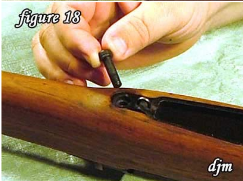
18) Remove the front trigger guard screw.
