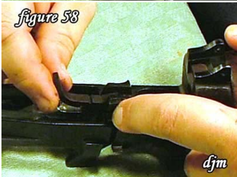
58) Set the bolt head catch plate in place.
