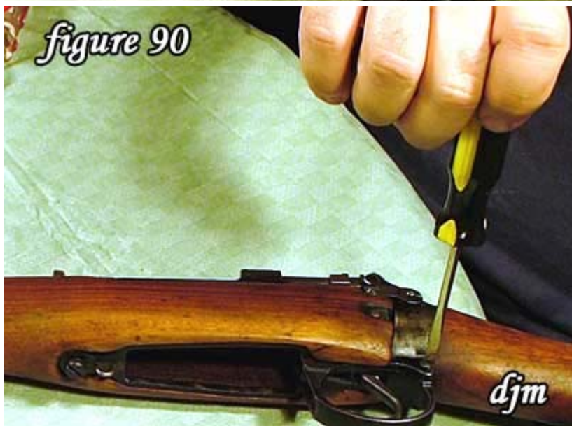
90) Tighten the rear guard screw.
