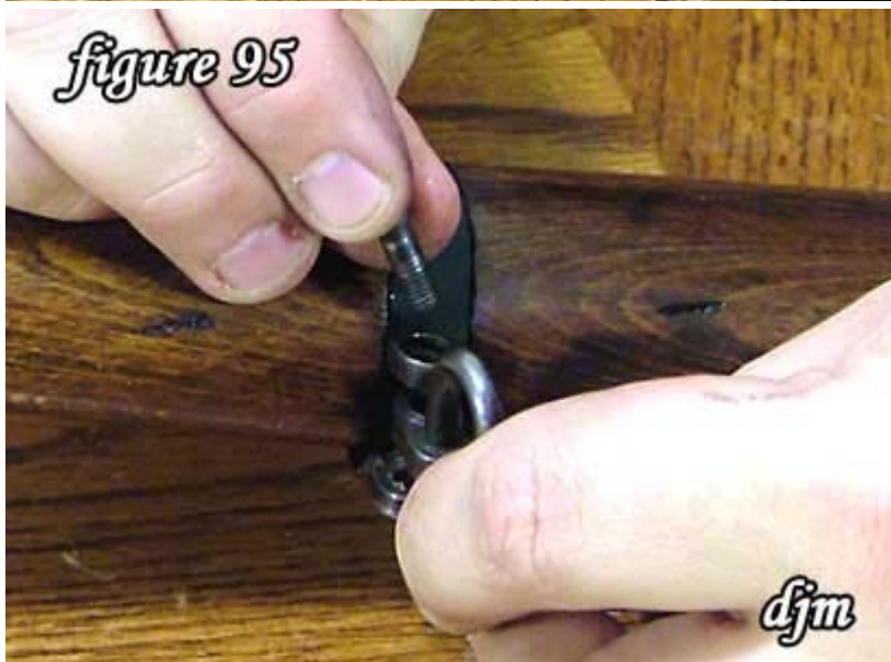
95) Replace the rear swivel screw and the sling swivel.
