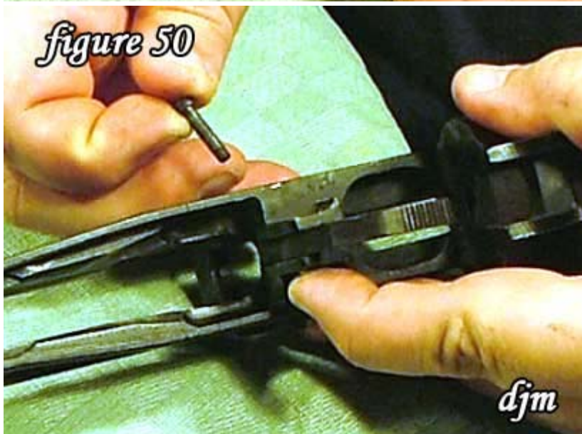
50) Remove the magazine catch screw.
