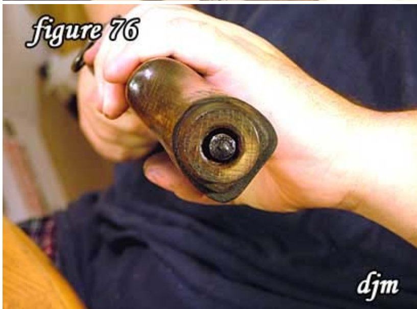
76) Figure 76 shows the front of the butt stock with the stock bolt protruding.
