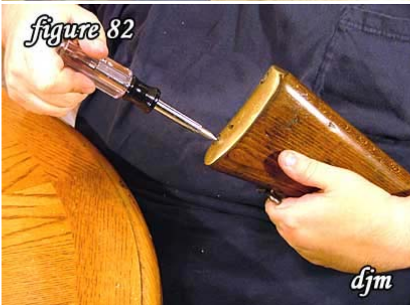
82) Figure 82 shows the correctly installed butt plate.
