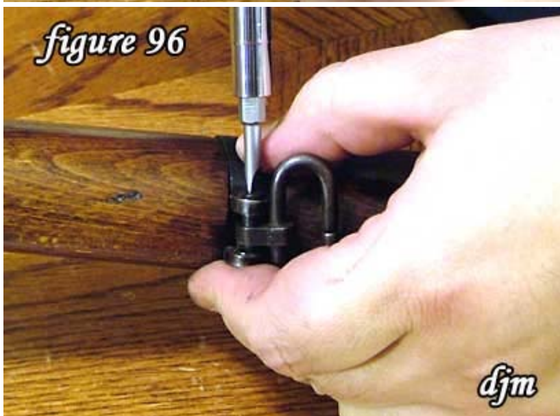
96) Tighten the rear swivel screw.
