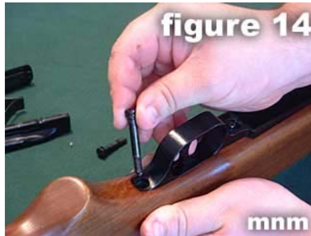
14) Remove the trigger cover rear screw .
