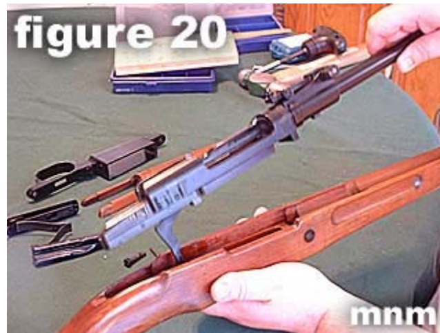
20) Place barrel and receiver assembly back into the rifle stock as shown in figure 20 .
