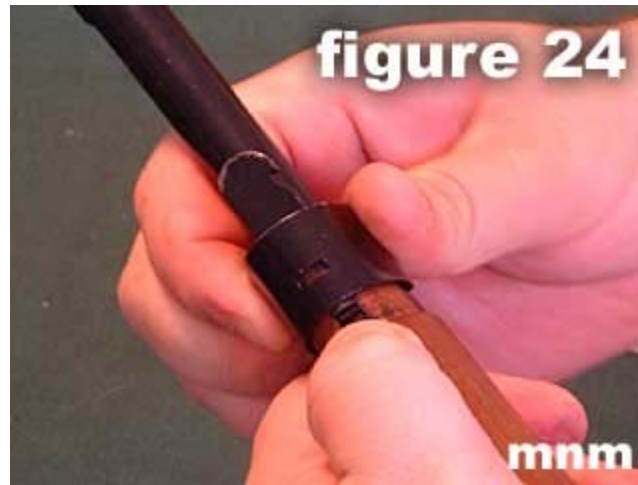
24) Depress retaining spring for the bayonet lug band as shown in figure 24 .
