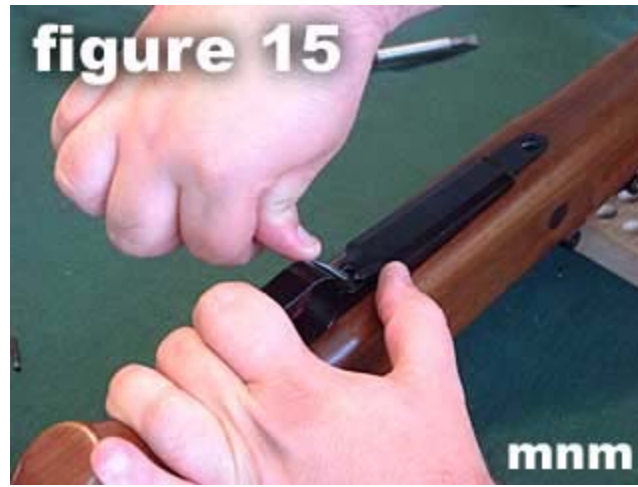
15) Press down on the magazine cover release and slide the magazine cover forward.
