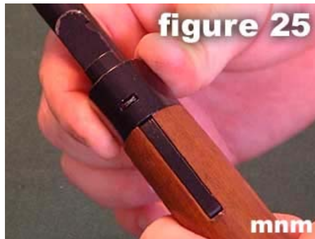
25) Slide the bayonet lug band until it locks in place.
