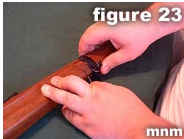
23) Depress the retaining spring and slide the lower barrel band till it is locked in place.
