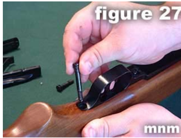
27) Install rear trigger guard screw.
