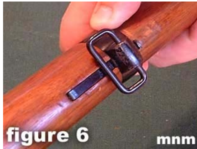
6) The lower band is also held in place by a retaining spring .
