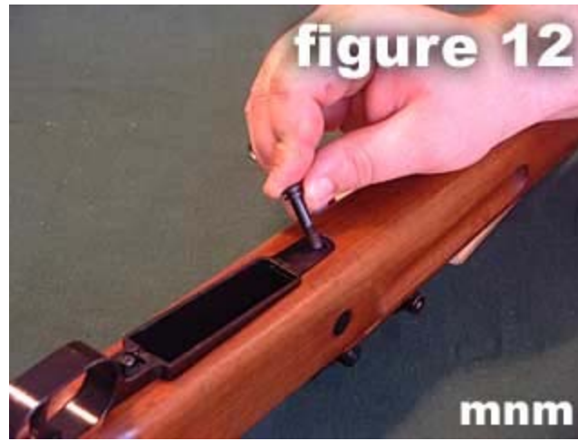
12) Remove the trigger guard front screw .
