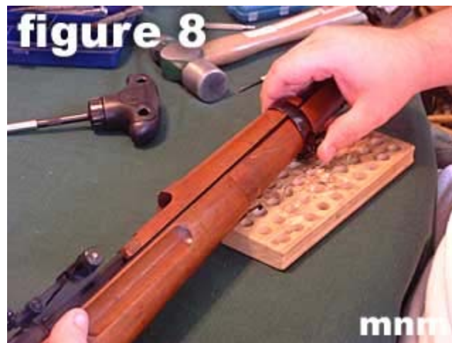
8) Remove the lower barrel band by sliding it forward. You will have to slide the handguard as well since it has a lip located at its front.
