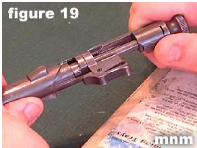
19) Figure 19 shows the lug of the safety locked into place inside the bolt .
