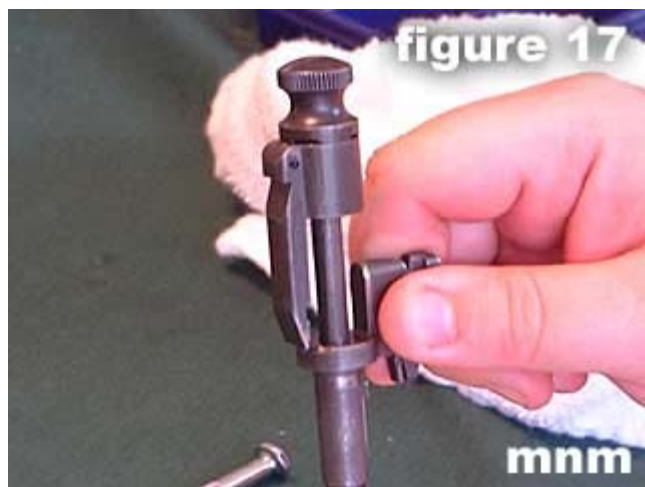
17) Turn cocking piece and sleeve and let sear contact lug rest on lip of safety (as shown in figure 17 ).
