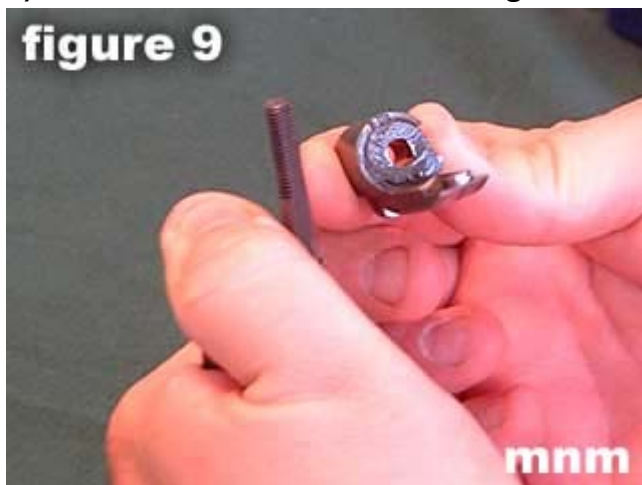
9) Note that sleeve/sear contact lug is keyed to striker (as shown in figure 9 ).
