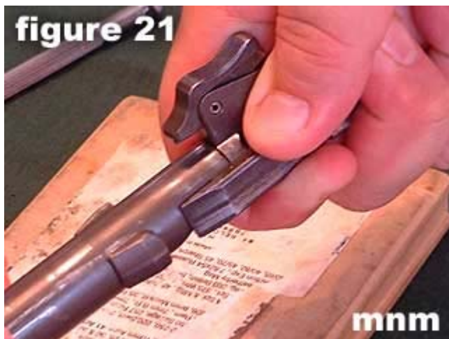
21) Pull and turn sleeve and cocking piece . Slide sear contact lug into channel on bolt (as shown in figure 21 ).
