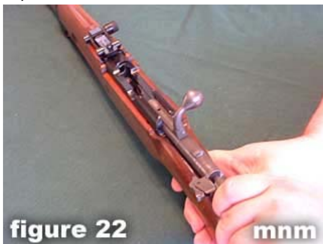
22) Depress trigger of rifle and return bolt to receiver.
