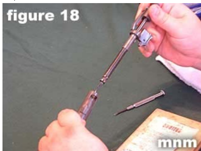
18) Return striker assembly to bolt and turn cocking piece either direction to lock lug into bolt .
