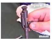
17) Turn cocking piece and sleeve and let sear contact lug rest on lip of safety (as shown in figure 17).
