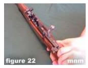
**22)** Depress **trigger** of **rifle** and return **bolt** to **receiver**.
