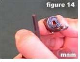
**14)** Align flat sides of **striker** with flat sides of **sleeve**.
