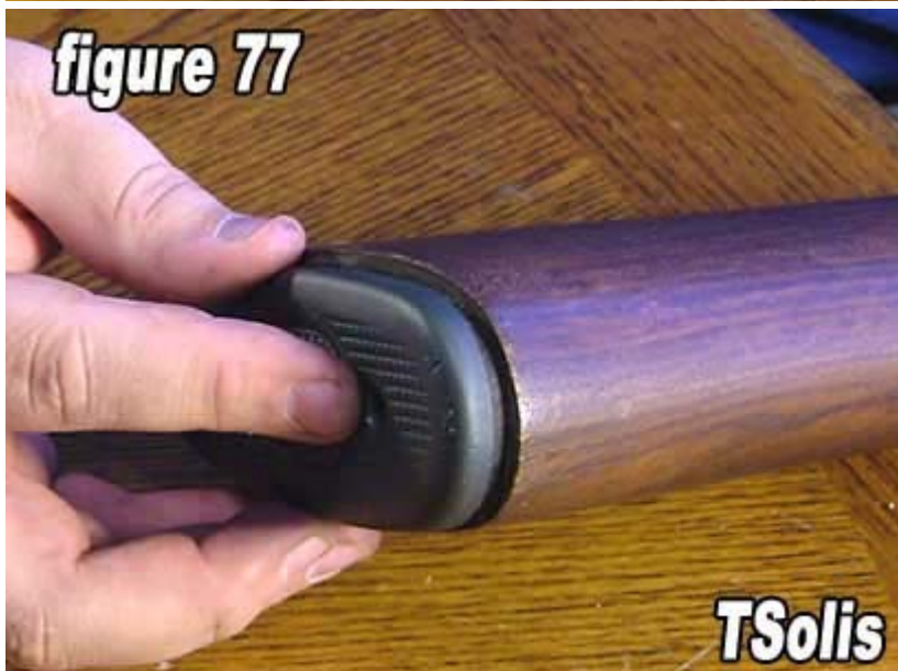
77) Install the butt plate assembly
