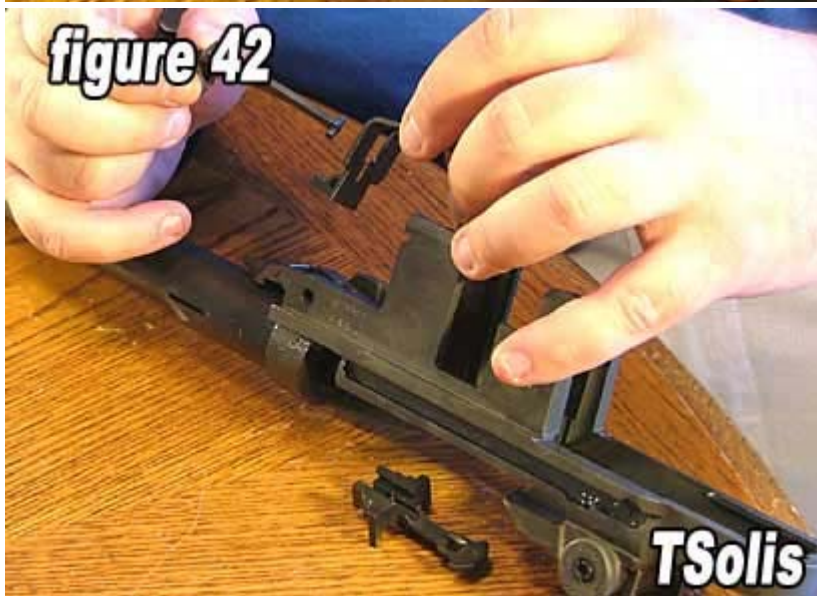
42) Lift out the follower arm and bullet guide. Note the follower and slide assembly slid out of the receiver.
