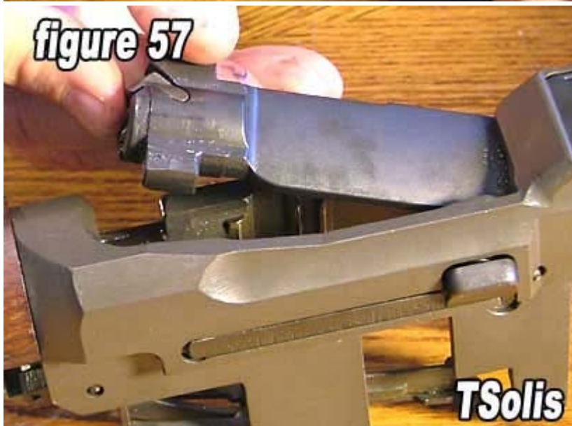
57) Pivot the bolt into the receiver as shown in figure 57.
