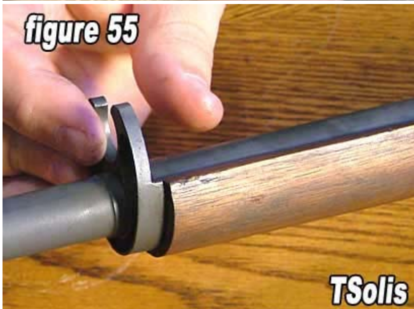
55) Slide the lower band till it mates with the lower hand guard.
