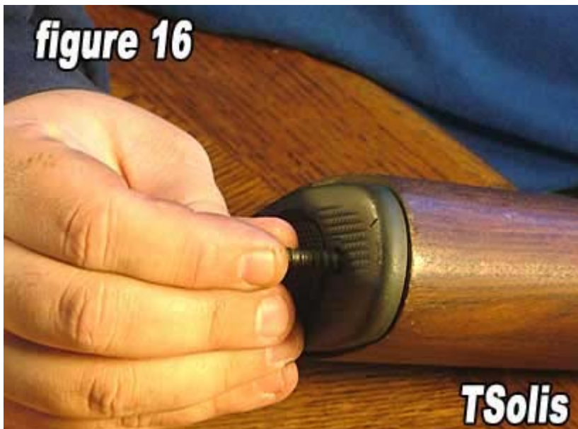
16) Remove the upper butt plate screw.
