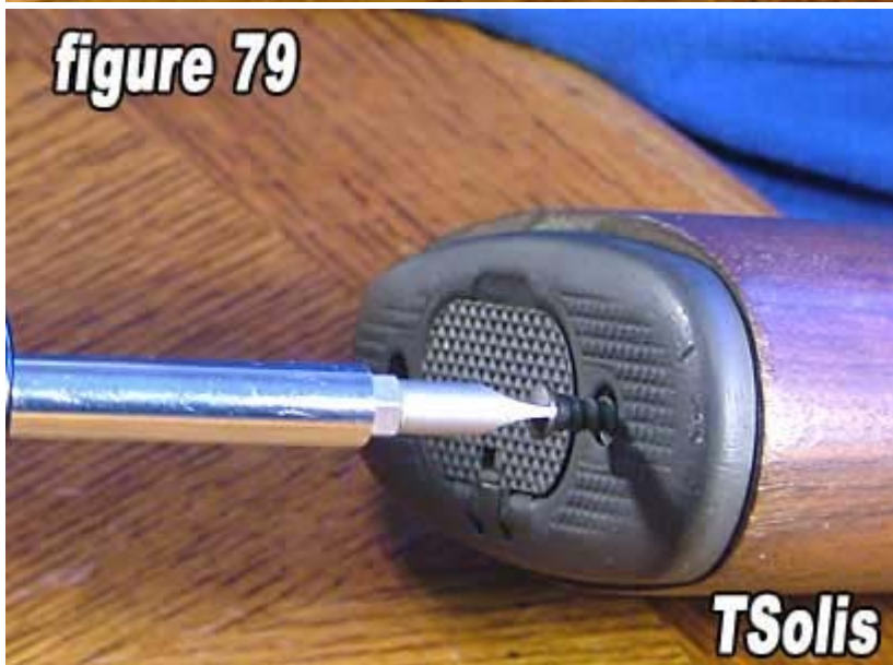
79) Tighten the upper butt plate screw
