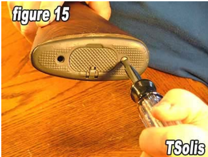
15) Unscrew the upper butt plate screw.
