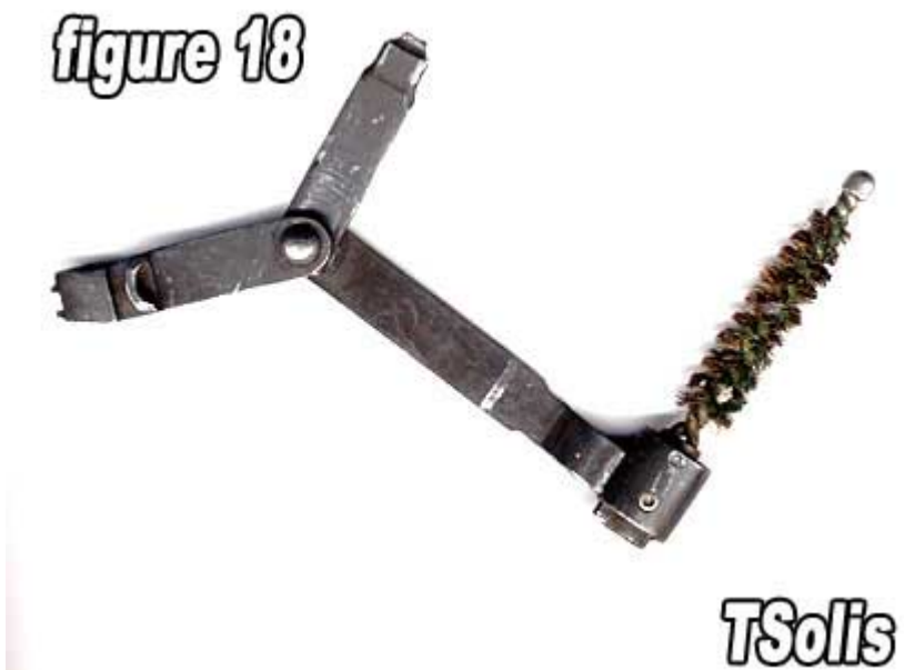
18) Figure 18 shows the M1 Garand Combination Maintenance Tool
