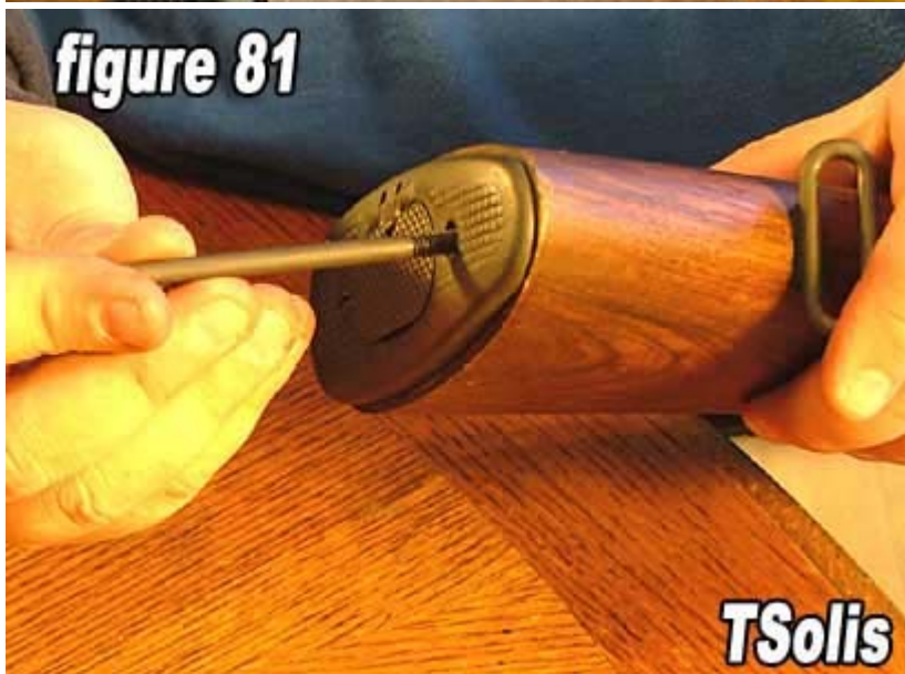
81) Insert the lower butt plate screw
