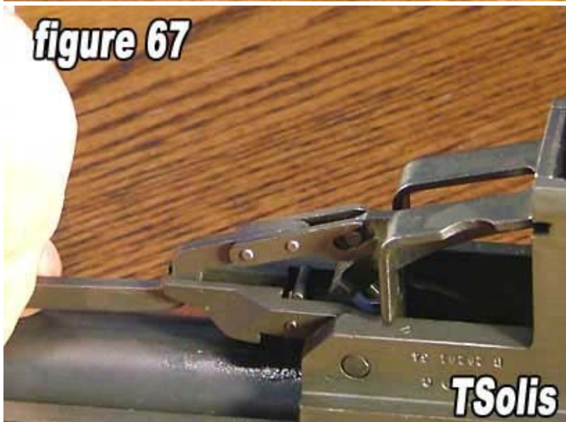
67) Figure 67 shows the correct attachment of the follower rod to the follower arm.
