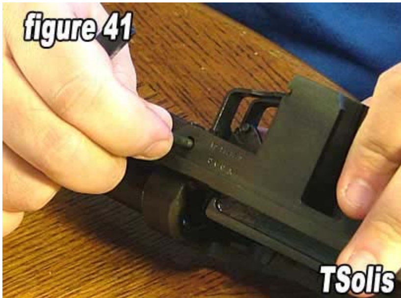
41) Pull the follower arm pin out the rest of the distance on the right side of the receiver.
