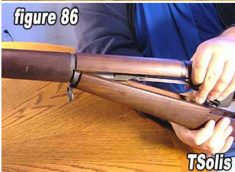
86) Pivot the assembled rifle upper into the assembled rifle stock as shown in figure 86.
