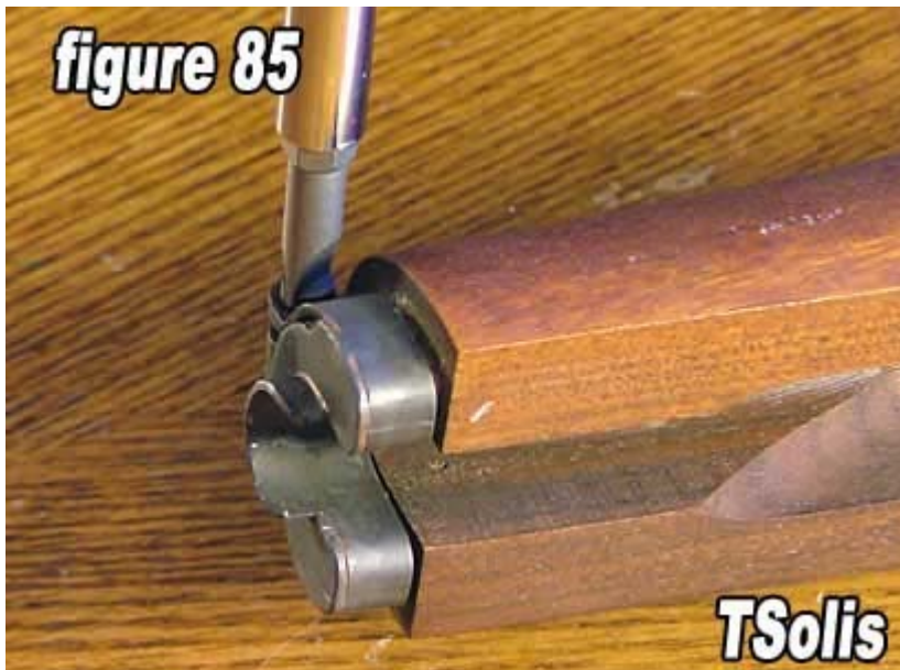
85) Tighten the ferrule swivel screw.
