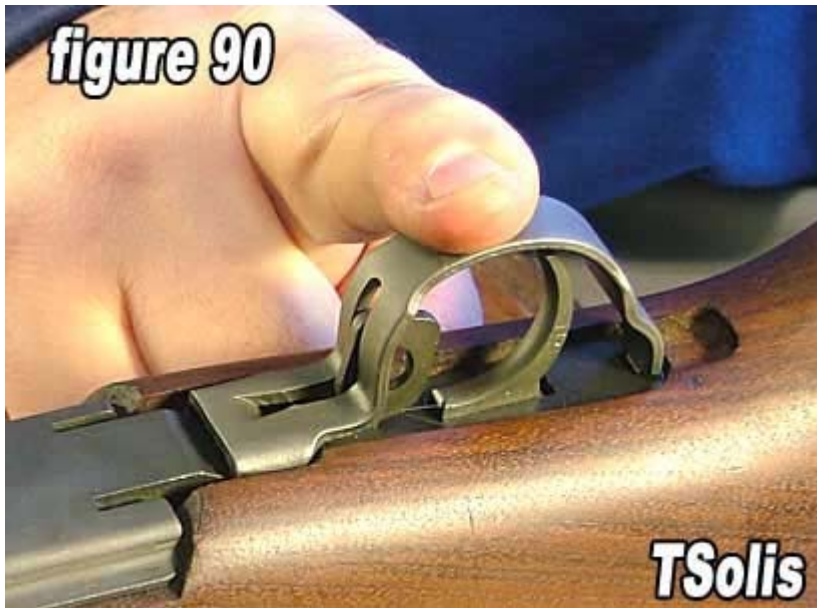
90) Lock the trigger guard in place.
