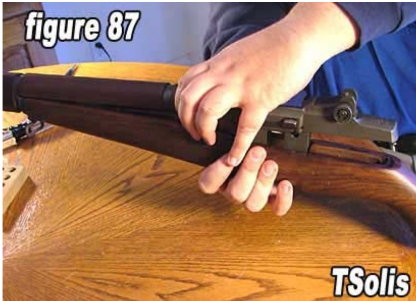
87) Insert the receiver into the stock.
