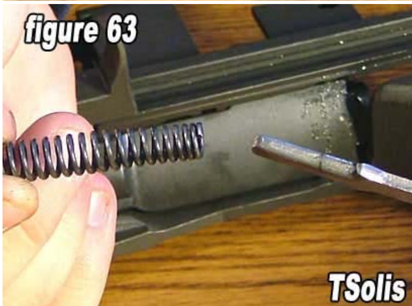
63) Note the tapered end of the operating rod spring as shown in figure 63.
