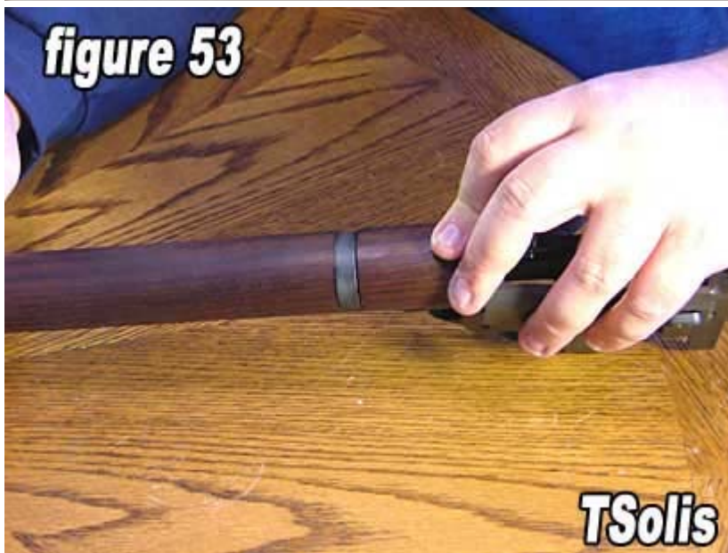
53) Snap the rear hand guard band clip into the grooves in the side of the barrel.
