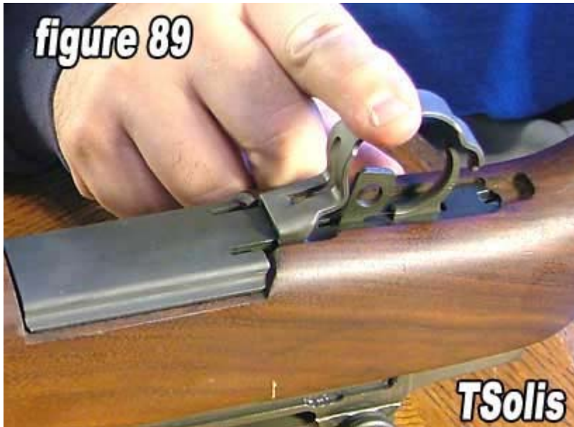
89) Rotate the trigger guard to the rear.
